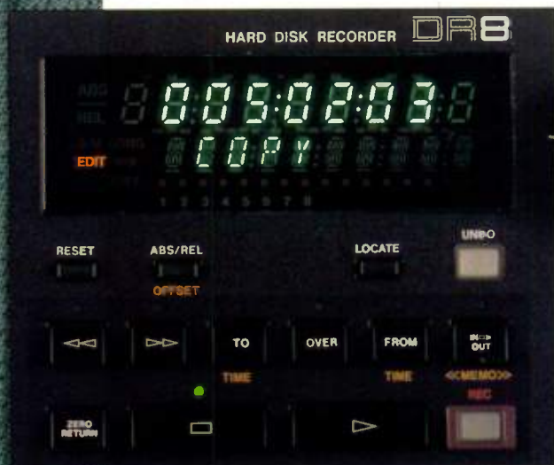
The DR8 uses familiar tape transport controls, whilst retaining all the advantages of a random access system.
