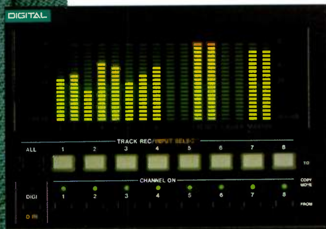
The large bargraph peak indicators display the individual levels of the eight hard disk tracks, as well as aux send levels, bus levels, and stereo master outputs.
