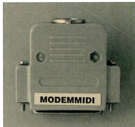
ModemMIDI and 16+ both offer an extra MIDI Out from the ST's serial port.
