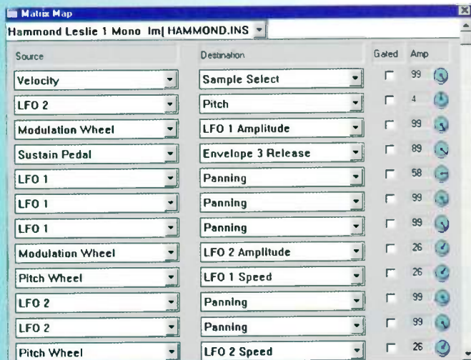
The Matrix Map lets you patch control signals to the sound generator, allowing a wide range of performance controls.
