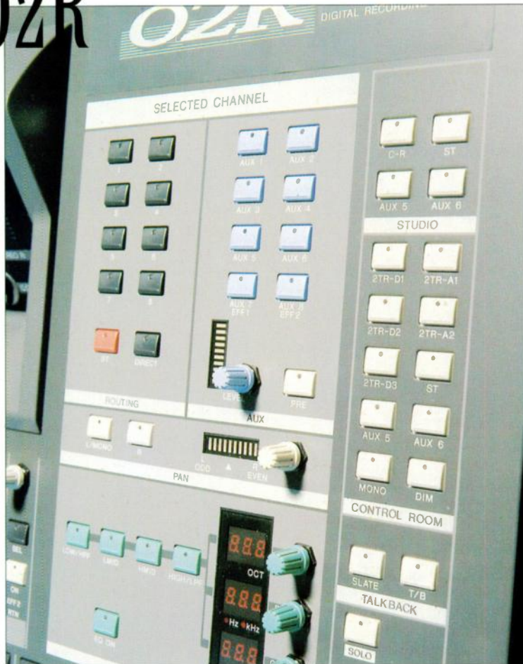
The Selected Channel controls provide direct access to routing, aux sends, EQ and panning for the currently selected channel.
