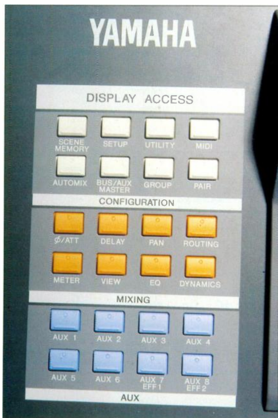
The Display Access panel — used to call up the numerous screen pages.
