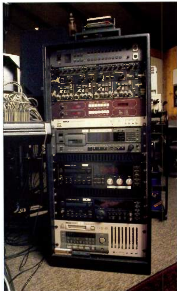
The effects and recording rack includes Alesis 3630 compressor, SPL Stereo Vitalizer, Optimizer, ARSonic Sigma 12, Tascam DA30, DA30 MkII, Tascam DA88 digital multitrack.
