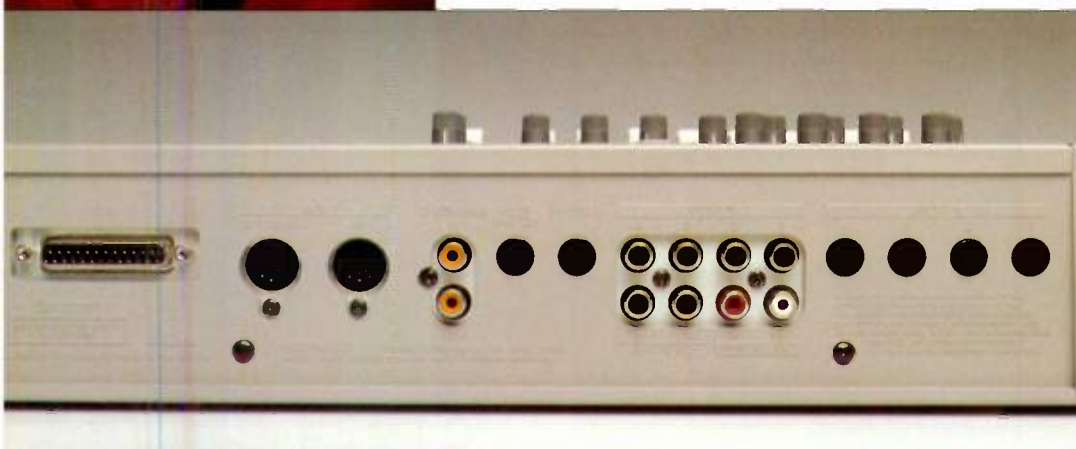
The back panel, featuring the all-important SCSI connector (left) for the attachment of external storage drives.
