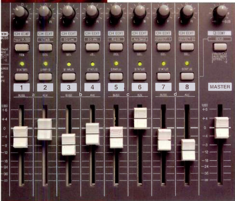
The mixer channel controls: physical controls access Pan and Level, but the EQ, effects and aux sends lurk behind the eight select buttons (under the Pan controls at the top of the picture).
