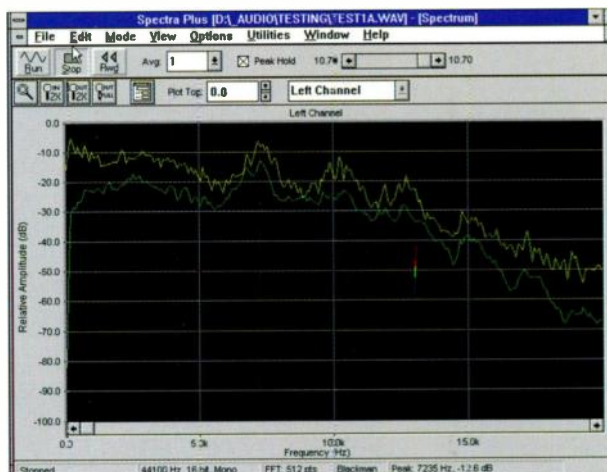
Using Spectra Plus, you can analyse the acoustic of a room. Here, the two traces show the off-axis and direct acoustic.
