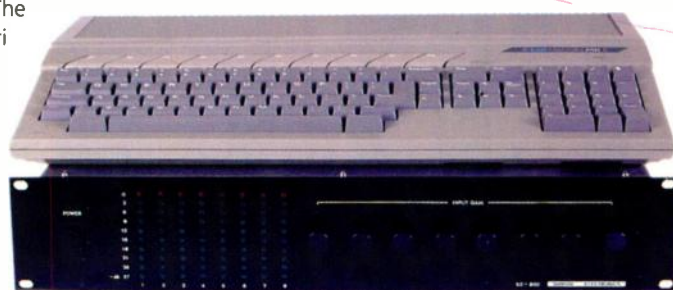
The SE800 adds 8 high-quality analogue inputs and outputs to the Falcon, with accurate metering and a flat frequency response.
