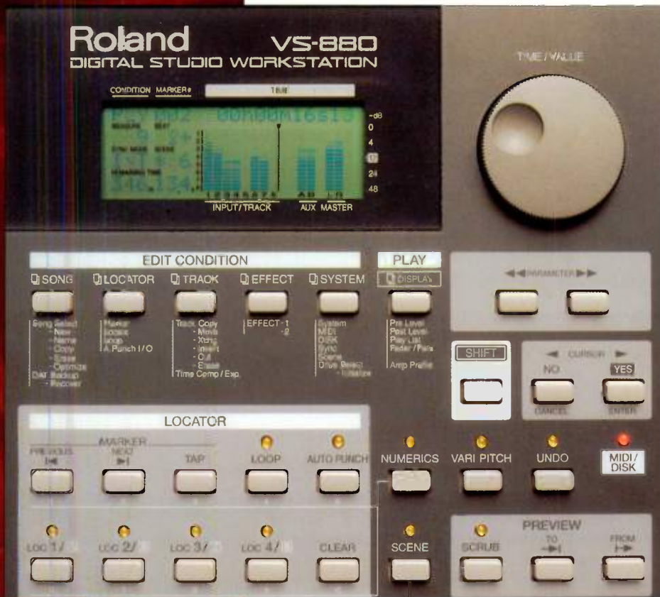
The LCD display, which changes readout depending on the mode selected using the buttons beneath.
