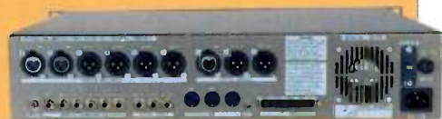
The back panel on the Pro version of the Soundscape hardware. Note the XLR analogue and AES/EBU digital ins and outs along the top.
