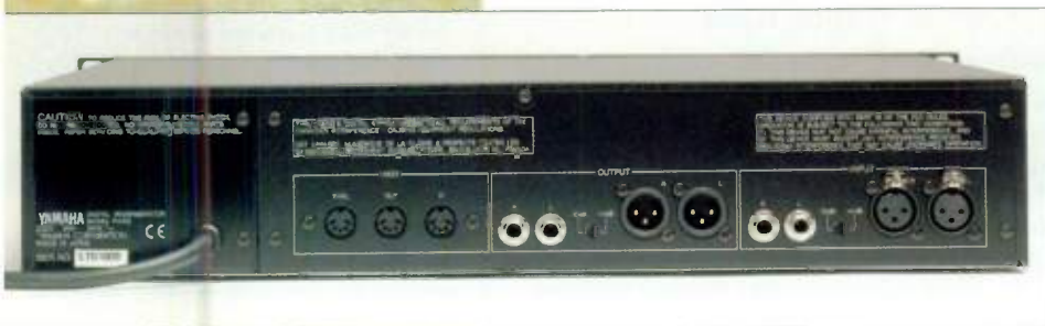
The Pro R3's back panel, helpfully offering XLR Ins and Outs alongside the jack sockets.
