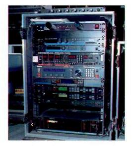
Cure rack shot number 2 — outboard including Lexicon PCM70 and PCM80 effects, TC Electronic TC2290 delay, Eventide H3500 UltraHarmonizer, Yamaha SPX1000, SPX900 and SPX90 MkII, and Roland Dimension D Chorus and delay.
