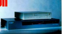
internal extras, including S/PDIF or ADAT digital interfaces, RAM expansion to 14.3Mb, 1Gb or 2Gb internal hard drive, removable drives, accelerator cards, and so on. The Falcon 68030-based Mk X will work with Atari Mega ST or Mega STe keyboards (the Mk X-AT allows you to use a PC keyboard), and it can be used with standard SVGA, RGB or ST monitors.
