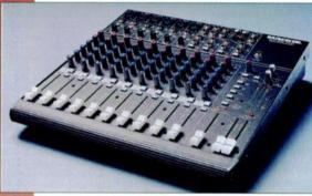
mic/line channels plus four stereo line channels and two stereo aux returns, the 1402VLZ has global phantom power, plus phono connections for a 2-track recorder. Each mic/line input has a switchable 75Hz, 18dB/octave low-cut filter, a gain Trim control and an insert point.
