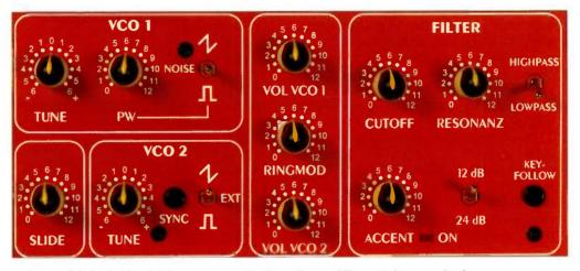
A close-up of the left-hand end of the ProTone, showing the oscillator and filter controls in more detail.
