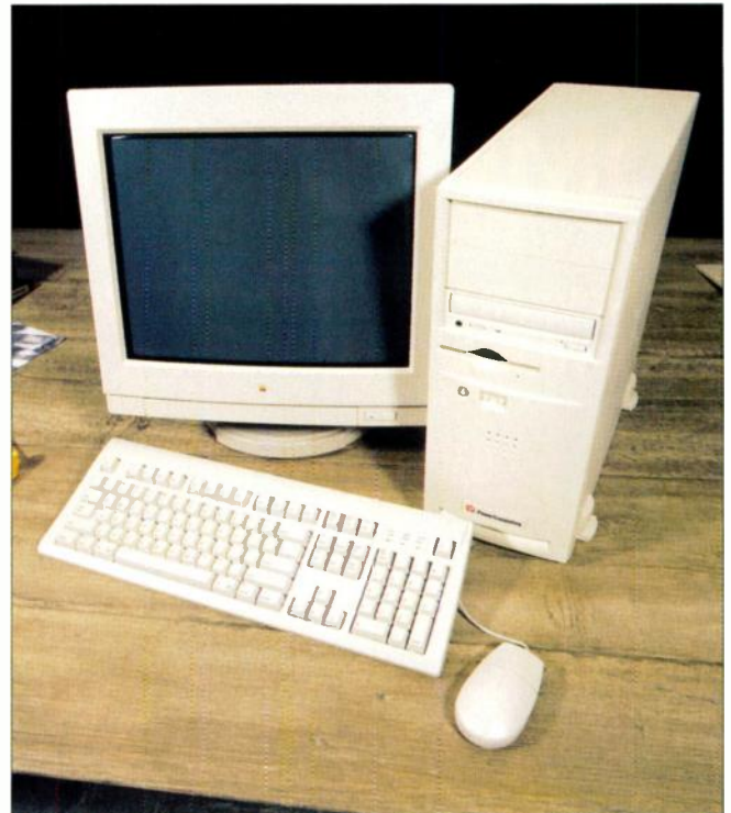
Power Computing's Mac clones (like the P120 pictured here) make worthy alternatives to bona fide Apple Macs — but be sure to check the clones' expansion slots if you're contemplating using your machine with a Digidesign system, as the newer models appear to be swapping from NuBus to PCI slots...
