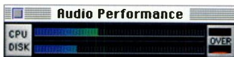
The Audio Performance window monitors the load on your CPU and hard disk.
