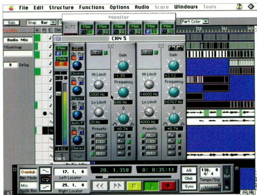
EQ setup window and effects sends: there are two EQs showing here, but you can have as many as four per channel if your system permits it. The 'Dry' button at the top of the effects send column kills all sends for that audio channel.
