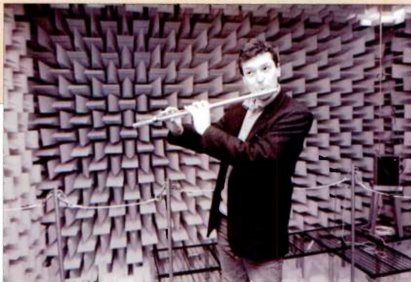
Symbiosis flautist John Hackett in an anechoic chamber at the BBC's Research Establishment at Kingswood Warren. The complete lack of reflections from the walls makes it very difficult to play, and shows how useful digital reverbs can be to create a good acoustic environment in the studio.
