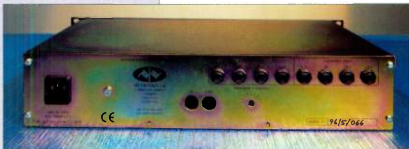
The basic Mutator's rear panel (although the MIDI version was tested for this review). This version also sports the inconveniently-sited rear panel MIDI channel selector.
