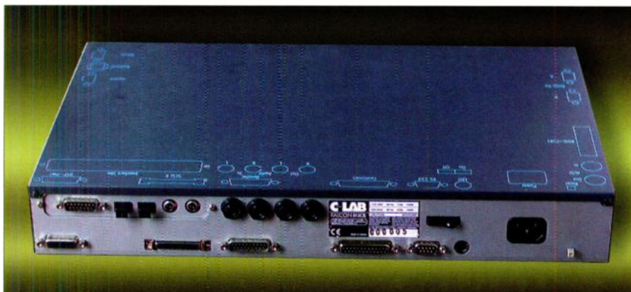
The optional S/PDIF interface is installed internally, with its ports accessible from the back of the machine. Note also the new quarter-inch jack sockets that replace the flimsy stereo mini-jacks of previous models.
