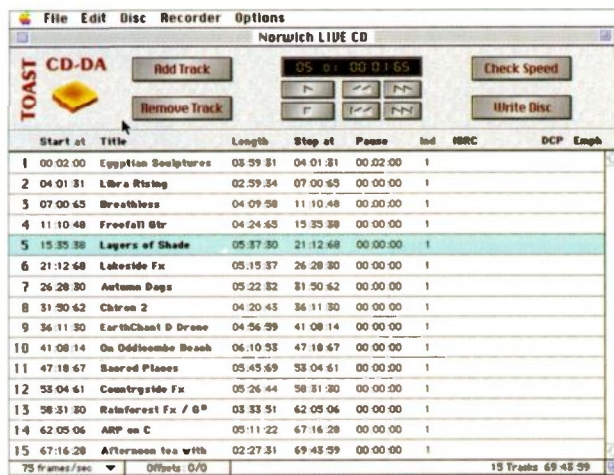
Figure 2: Symbiosis use Astarte's Toast CD-DA software (see page 148) to burn CDRs complete with the PQ encoding necessary for glass mastering. P codes tell the CD player when audio data is present, while Q codes describe the track and disc running times, copy prohibit, emphasis and catalogue information. These codes are not added by a normal audio CDR recorder, so you have to use a computer-based CD-ROM writer with software like Toast for your disc to be a suitable master to work from. Toast recognises Sound Designer II files and regions, so you can set track indexes in the middle of segued music if you divide it up into regions in Sound Designer first!
