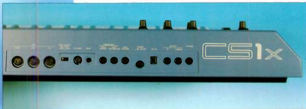
The CS1x's rear panel connections, including the PC/Mac interface.
