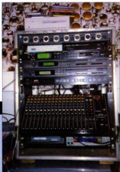
Live 'Star: this rack is the heart of the band's setup, both in the studio and on stage, and includes their Roland S760 sampler, Korg Wavestation SR, M3R and Yamaha TX81Z synth modules, Tascam MM1 keyboard mixer, and Alesis Midiverb and Zoom 9030 effects.
