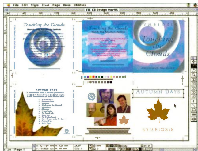
Figure 3: This screenshot from the Mac shows the full-colour artwork from two Symbiosis CDs assembled on a desktop publishing package. The page, which is slightly larger than A3 size, includes cut and fold marks, printer's colour bars, and cross-hairs for registering the four separate plates that will be used to print the Cyan, Magenta, Yellow, and Black inks.
