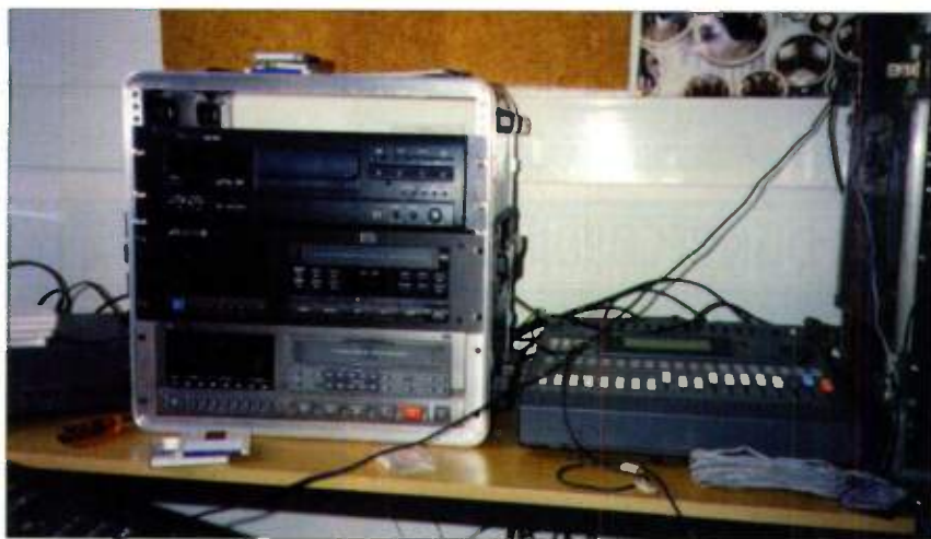
Dubstar record non-MIDI instrumentation and vocals on their Alesis ADAT (middle) and ADAT XT (bottom left), merge it with the backing from their MIDI instruments in the Yamaha ProMix 01 digital mixer (bottom right), and master the results with their Tascam DA20 DAT (top left).
