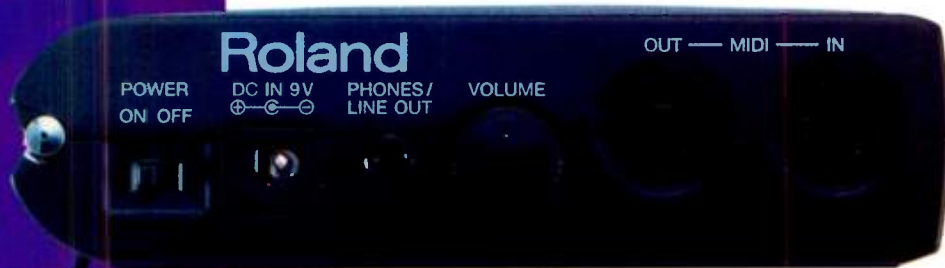
The PMA5's rear panel. The computer port is out of sight on the side of the unit. But if you can use the PMA5 as a MIDI interface, why is there no MIDI Thru socket?
