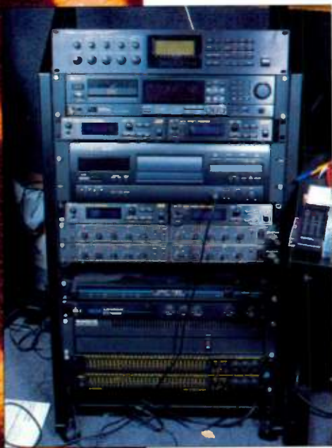
The recording rack, including: Roland E660 digital EQ, Sony DTC1000 DAT, a Tascam DA20 DAT sandwiched between two Boss SE70 effects processors, and two Drawmer LX20 compressors.
