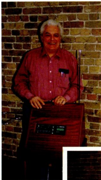
Bob Moog's 'deluxe', mahogany cabinet MIDI theremin. Like the standard model (inset) it has two antennas, one for pitch and the other to generate a control signal, usually for amplitude.
