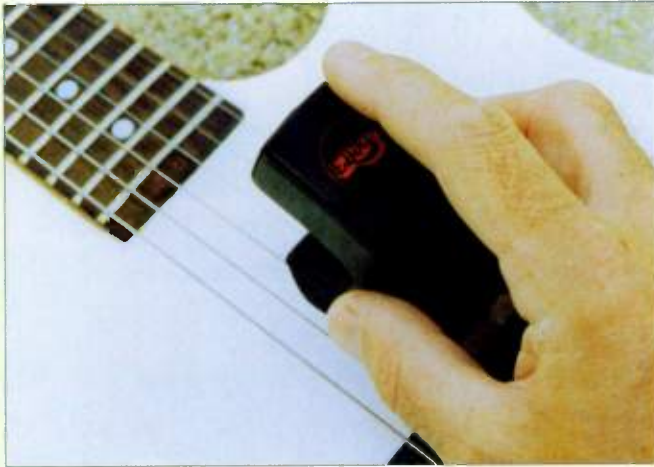
An e-bow can considerably extend the tonal palette of your electric guitar, yielding some fascinating, almost synth-like evolving tones.
