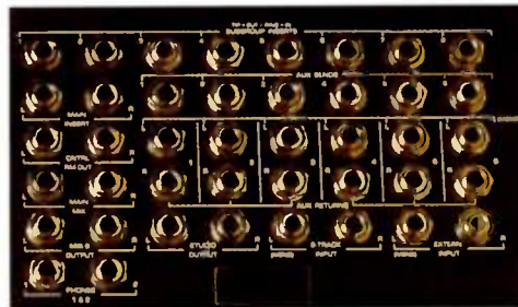
Typical rear panel of a mixing desk showing Aux returns and channel Insert points.
