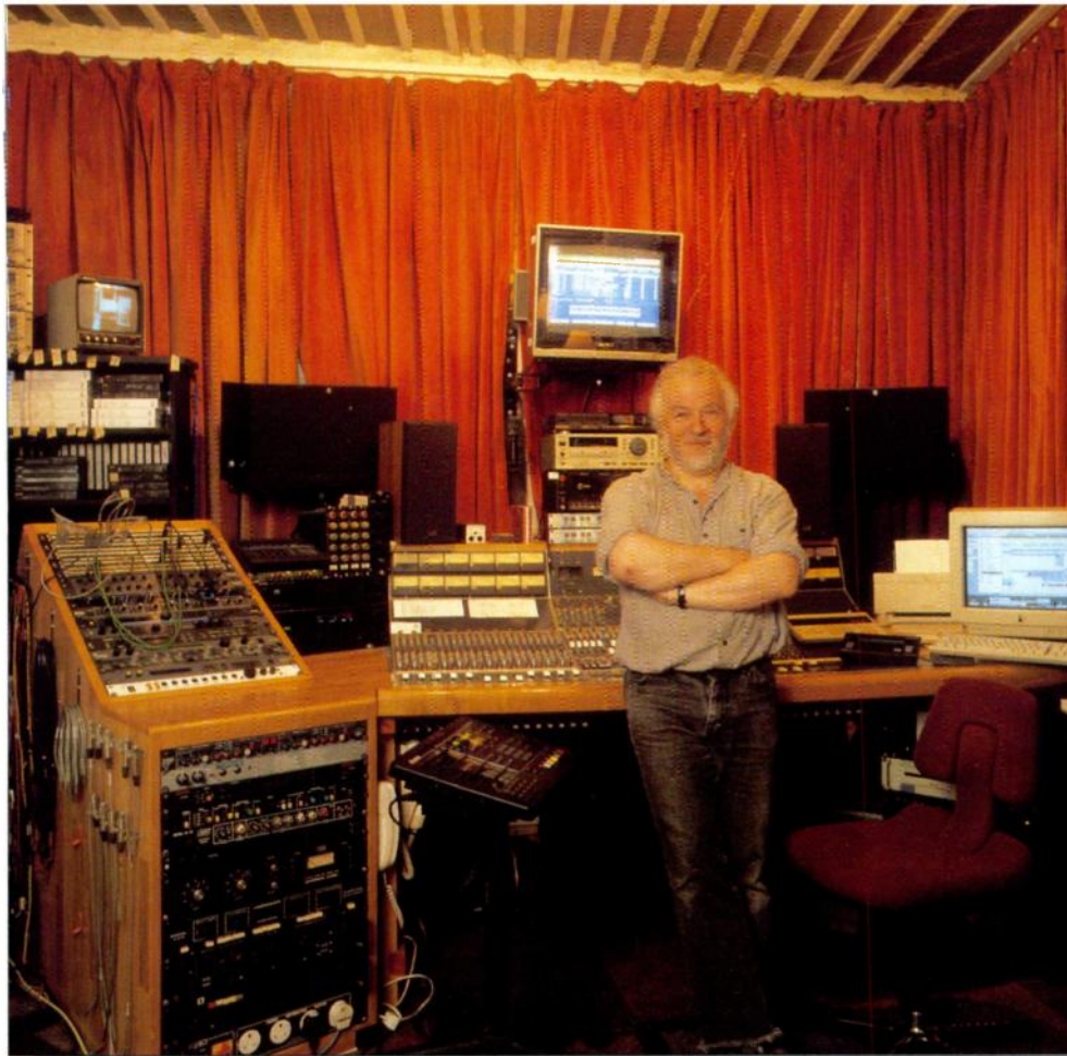
David's comprehensively-equipped Terra Incognita control room. The three ADAT XT's used for the bulk of the recording work can be seen to the far left, on top of the tall shelf unit. The BRC remote sits by the mixing desk for easy access. The Mac computer, to the right of the desk, runs Cubase Score software, and the display to the centre of the photo helps David to get the best out of his Roland S760 sampler — when he's not using the screen for his picture work. David's favourite signal processor, the TC Electronic M5000, lives in the rack under the main work surface, to the right.
