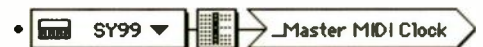
Figure 2: The Studio 5LX's filter block (between the SY99 and Master MIDI Clock) filters out everything coming from the SY99 other than MIDI clocks and related messages, in this Virtual Controller.
