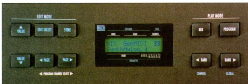
The QS8's display, with Edit and Play Mode buttons to either side.
