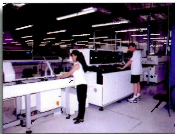
Mackie's High Speed Surface Mount Line, incorporating a Panasonic Chip Shooter that places approximately 30,000 parts per hour.
