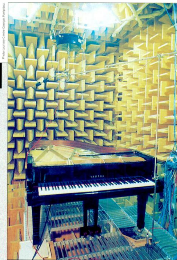
The Anechoic Chamber.
