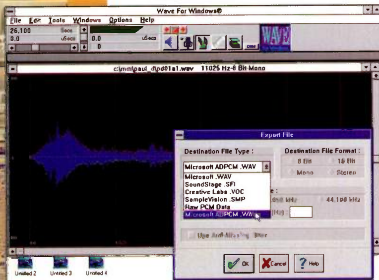
Wave editing software (such as Wave For Windows, shown here) will usually be able to export recorded audio data in various formats, allowing sample rate and format conversion.
