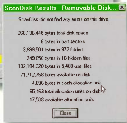
Microsoft ScanDisk in action. This is the result for a SyQuest 270Mb drive — notice that for a drive of this size, each allocation unit (or cluster) is 4K in size.
