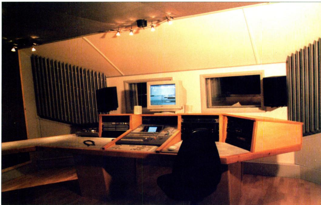
This 02R/SADiE production room at LBS, Stockport is further simplified, but still benefits from its diffusive front end.
