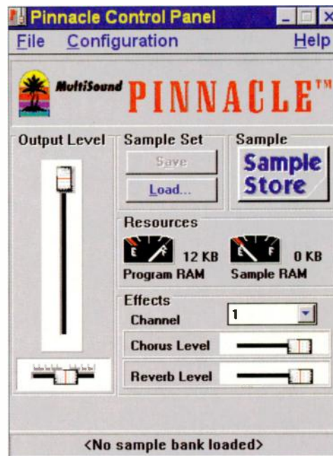
The Pinnacle's control panel — used to load user sample banks, set overall output levels, and manually adjust effects for each MIDI channel.
