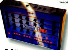
marketing company Global Distribution have taken on UK distribution of the German-built JoMox Xbase09 drum machine. Based on MIDI-controlled analogue circuitry, the Xbase09 produces three instruments — bass drum, snare and hi-hat — all under real-time MIDI control. The sounds can be drastically altered, in real time, including reverse
