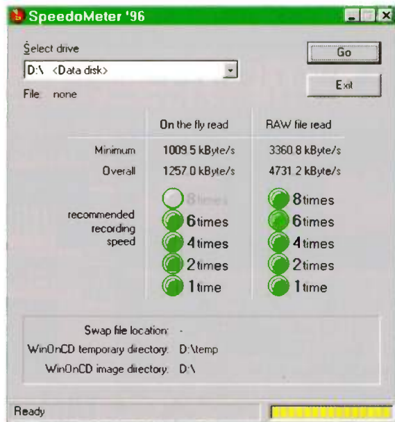
Figure 4: Supplied with the latest version of WinOnCD 3.0, the SpeedoMeter gives your system speed a series of tests to determine how well the rest of your system will perform.
