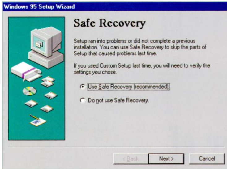
Figure 5: If your machine crashes during the installation of Windows 95 itself, you need to run Windows 95 Setup again, and it should detect that you had a previous problem, bringing up this screen. Use Safe Recovery as shown here, and everything should complete with no further mishaps. If not, try the same procedure again.
