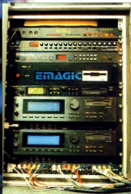
A mixed rack containing both sound sources (Oberheim Matrix 1000 and Novation BassStation rack), and samplers (Roland S750, S760 and S770).
