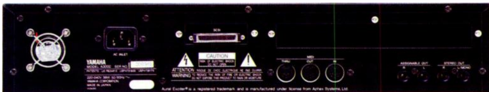
The A3000's back panel. The included SCSI connector is standard on all UK A3000s. The slot on the right is for the optional AIEB1 I/O expansion board.
