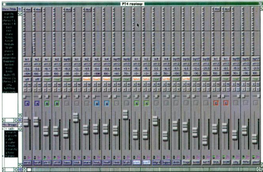
Faders can be displayed at half-width, allowing twice as many to fit on a screen.
