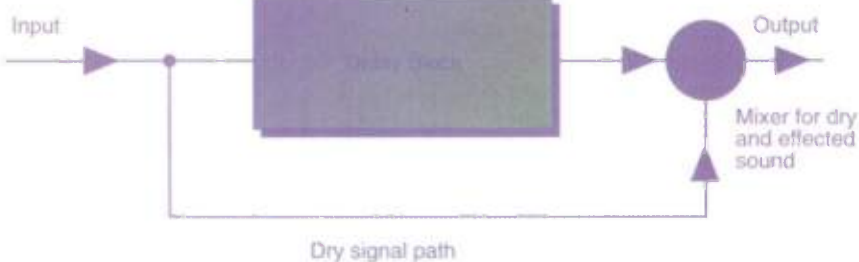
Figure 1: Delay block with wet/dry mixer.
