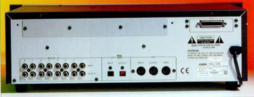
The D90's back panel, now with built-in ADAT interface. This unit has the SCSI option fitted (top right).
