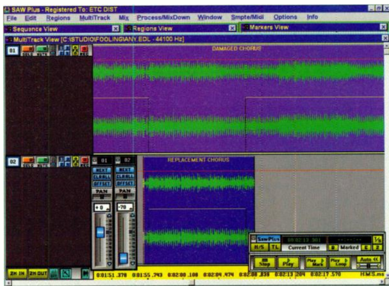
It is easy to replace regions of damaged audio material with material from elsewhere in the recording, using a multitrack editor like SAW Plus, by performing virtual splices — level-switching in real time between audio regions on adjacent tracks.
