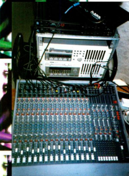
The core of James' new recording system; two Tascam DA88s, two Yamaha SPX90 effects units, and an Allen & Heath S2 mixer.
