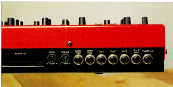
The Nord Lead 2's rear panel, including PCMCIA slot.
