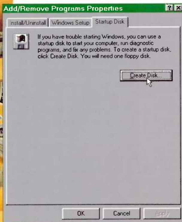
Figure 1: Don't pull out your old hard drive until you have created (and tested) a floppy startup disk. Once your new hard drive is in position and wired up, you'll need several of the small utility programs on this floppy to format and partition it.
