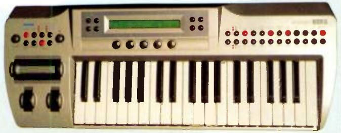
Korg's Prophecy keeps the FM flag flying to an extent with its VPM synthesis — effectively 2-operator FM.
