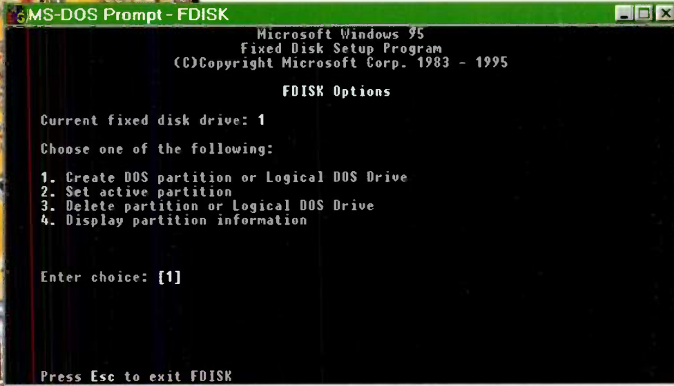
Figure 2: The charming text-only FDISK program, which you will find supplied with DOS or any version of Windows, and which you will need to run to partition your new drive. Your startup disk will also include this file.
