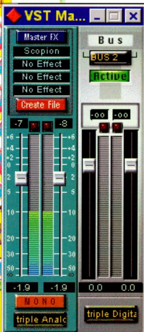
Figure 7: Up to four effects modules can be patched into the Master output, and multiple I/O cards can be used to provide an external buss to outboard processors.
