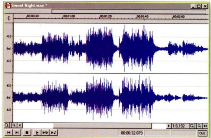
Figure 3: After normalising the track, the average level is significantly higher compared to the file shown in Figure 1 — with no compression, distortion, or other gimmicks.
