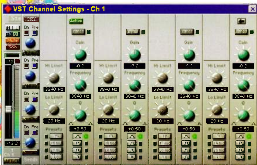
Figure 6: Each Audio channel may have four effects sends and four parametric EQs.
