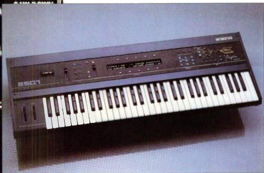
Ensoniq's ESQ1 was an early synth that featured short on-board PCM samples.
