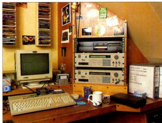
Morcheeba's computer and sampling setup — Atari 1040STFM running Cubase , two Akai S950s, and TEAC CD player.
