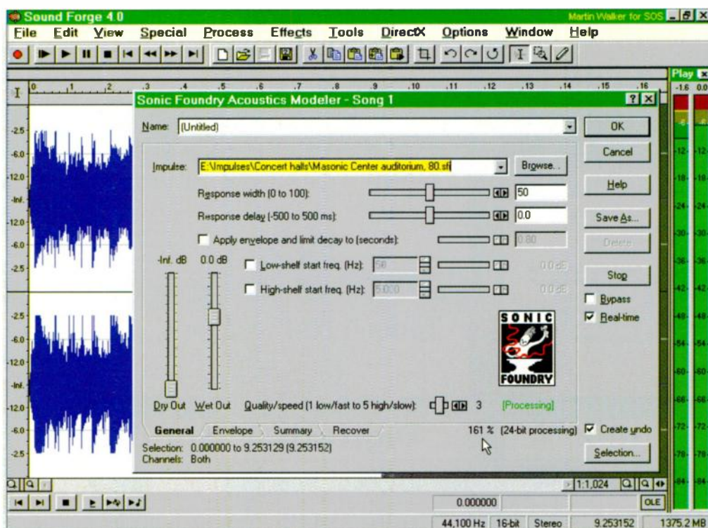
Here is the Acoustics Modeler window inside Sound Forge. The auditorium sound currently running in real time takes more than 100% of the computer's processing power with a Pentium 166MMX — but who said realism was easy?
