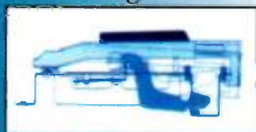
The Studiologic Key/Hammer assembly at rest.
