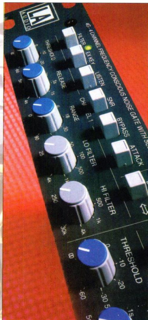
Stand-alone gates like the 4-channel LA Audio 4G (above) and the dual-channel Drawmer MX30 (below) can be most useful in reducing spill between miked-up drums.
