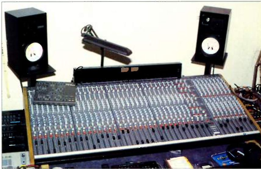
Left: Ola's Allen & Heath Spectrum desk, and Yamaha NS10M monitors. The Roland PG800 programmer is sitting on the top left corner of the desk.
