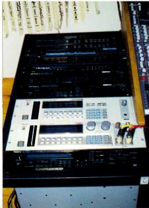
Above: (top-bottom): Yamaha SPX900, two Alesis Quadraverbs, Lexicon PCM70, and Digitech Studio 400 effects, Oberheim Matrix 1000 synth, Roland MKS70 and MKS20 synth modules, Akai S1000PB and S1000 samplers, and Roland JV1080 synth.
