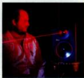
Mackie acoustic engineer David Bie uses scanning laser vibrometry to map HR824 tweeter dome vibrations.
