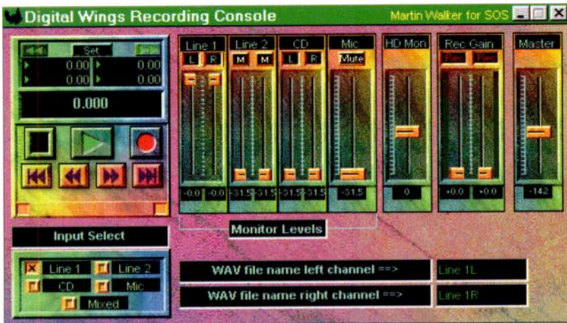
Figure 2: The Recording console provides a familiar graphic soundcard mixer interface, along with a comprehensive transport bar.
