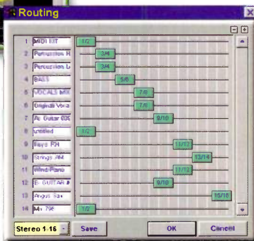
Below: Any of the 256 virtual tracks can be routed to any of the 16 physical output channels.
