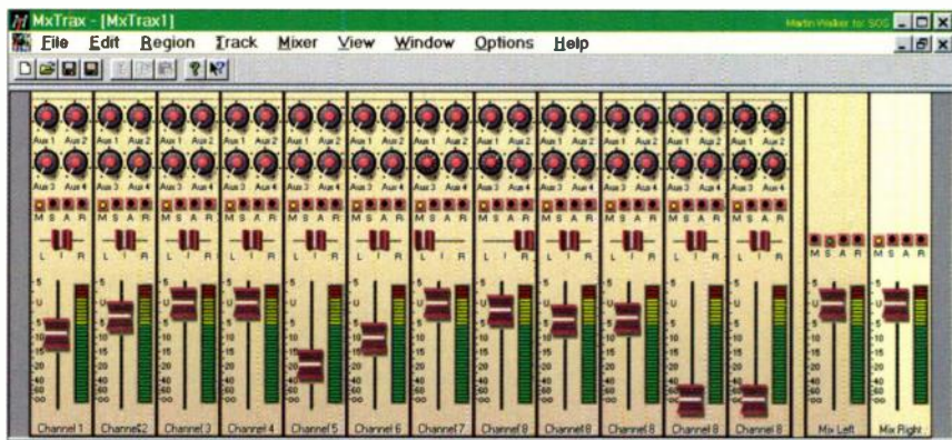
Above: The mixer in MxTrax is fully configurable, and even Automation is available, which allows fader and pan control movements to be recorded and played back.
