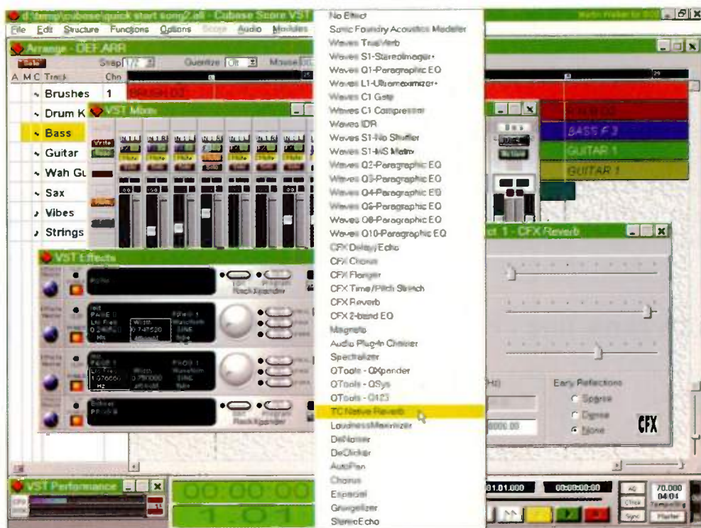
It's amazing how many effects can be crammed into a DMSS-compatible application like Cubase VST. Up to four different effects can be used for input channels, and four more as Master effects.
