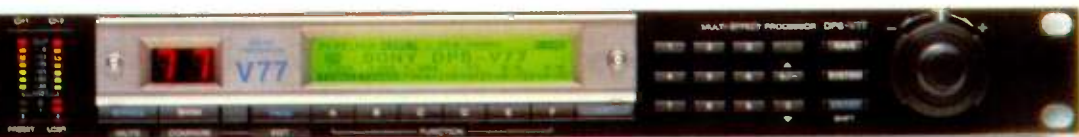
The Sony DPS V77 is just one of a number of effects processors that provide full digital I/O, so that you can preserve your digital path when adding external effects.
