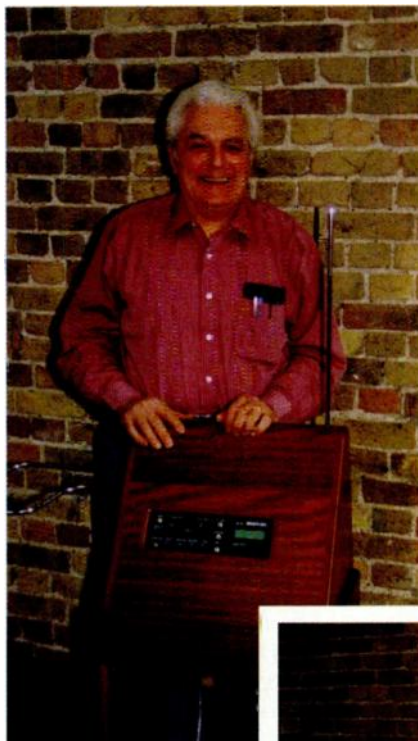
Bob Moog's 'deluxe', mahogany cabinet MIDI theremin. Like the standard model (inset) it has two antennas, one for pitch and the other to generate a control signal, usually for amplitude.
