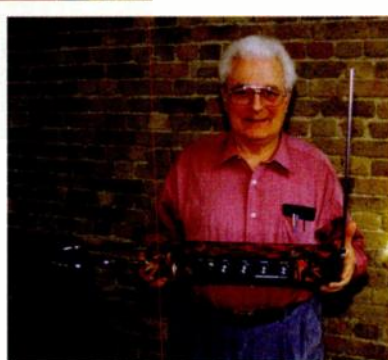
Bob Moog's 'deluxe', mahogany cabinet MIDI theremin. Like the standard model (inset) it has two antennas, one for pitch and the other to generate a control signal, usually for amplitude.
