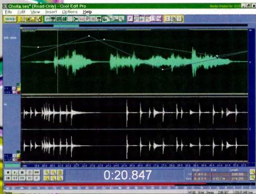
Figure 3: This zoomed-in waveform in the Multitrack View shows the volume and pan envelopes, while the three small coloured buttons to the left of the waveform control Mute, Solo, or Record Enable for each track. You can also see the stereo level meters at the bottom of the screen.
