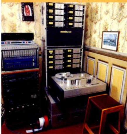
The Studer 2-inch 16-track is a converted 1-inch 8-track from 1969. Hedges prefers the sound of it at 15ips with Dolby A.
