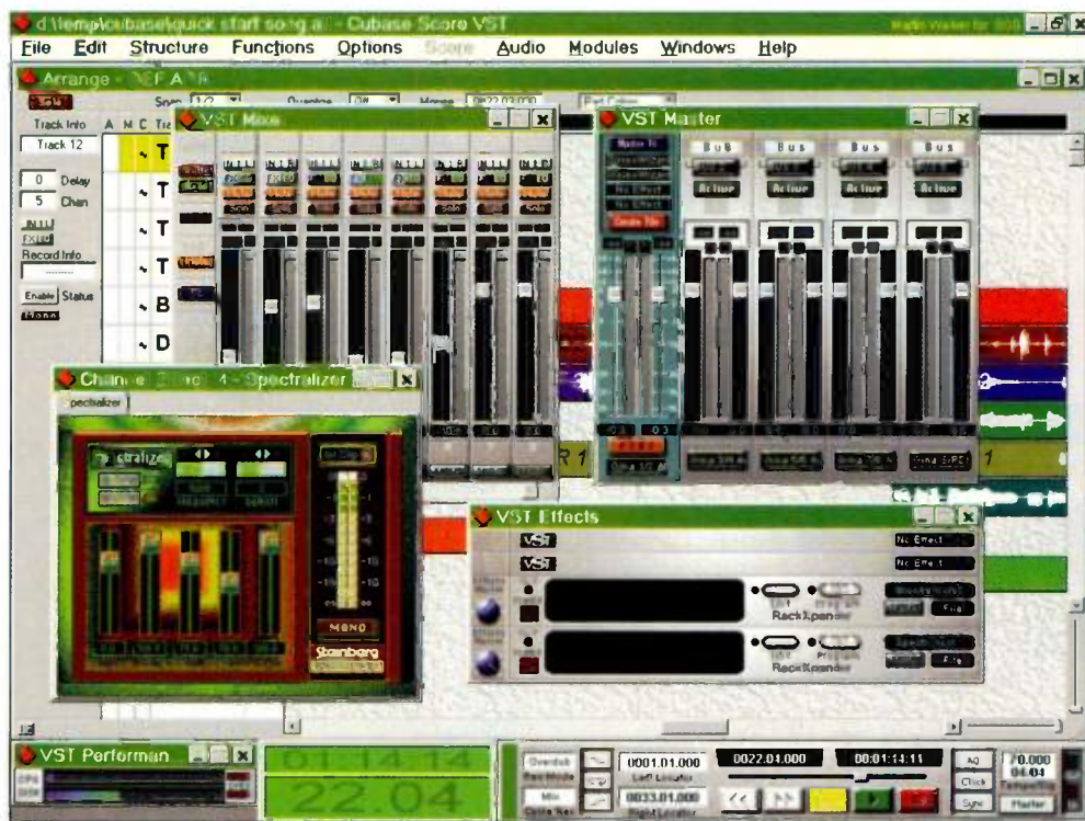
Figure 2: Here is an example of palette switching in action when using a display featuring only 256 colours. Since Steinberg's Spectraliser uses a completely different palette of 256 colours from that of Cubase VST, its colours look 'garbled' when VST is the active window.
