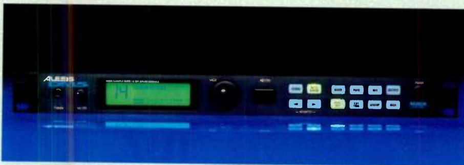
A more modern drum unit like the Alesis DM5 could help expand the MIDI potential of an older unit like the Yamaha DD11 no end... without the need to throw away the DD11 itself!
