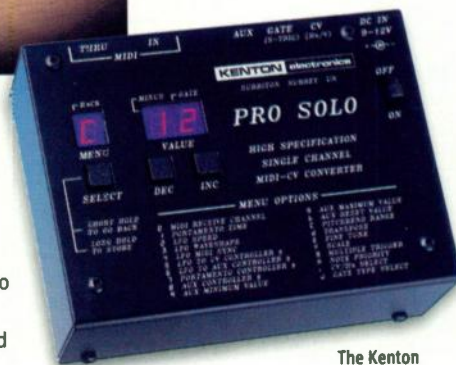
The Kenton Pro Solo is a versatile single-channel MIDI-CV converter and works with almost any monosynth (see page 82).
