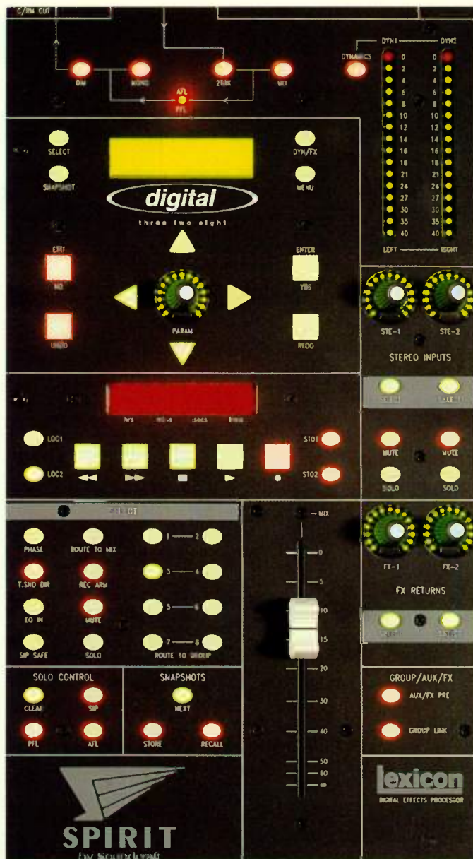
Because there are no menus to navigate, the 328 has only a two-line LCD display.
