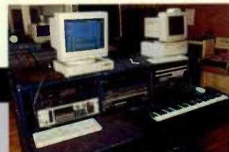
The programming station in Instrument Studio 1: Apple Mac Quadra 610, Emu E6400 and Akai S1100 samplers, Roland JV1080 synth, (next rack) Novation BassStation and DrumStation racks, patchbays, and an Apple PowerMac 7100.
