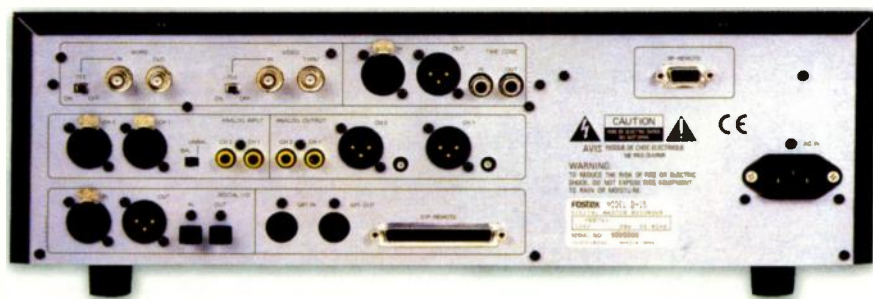
Not many mid-price DAT recorders offer word sync connections — this Fostex D-15 is an exception (see BNCs at top left of rear panel).
