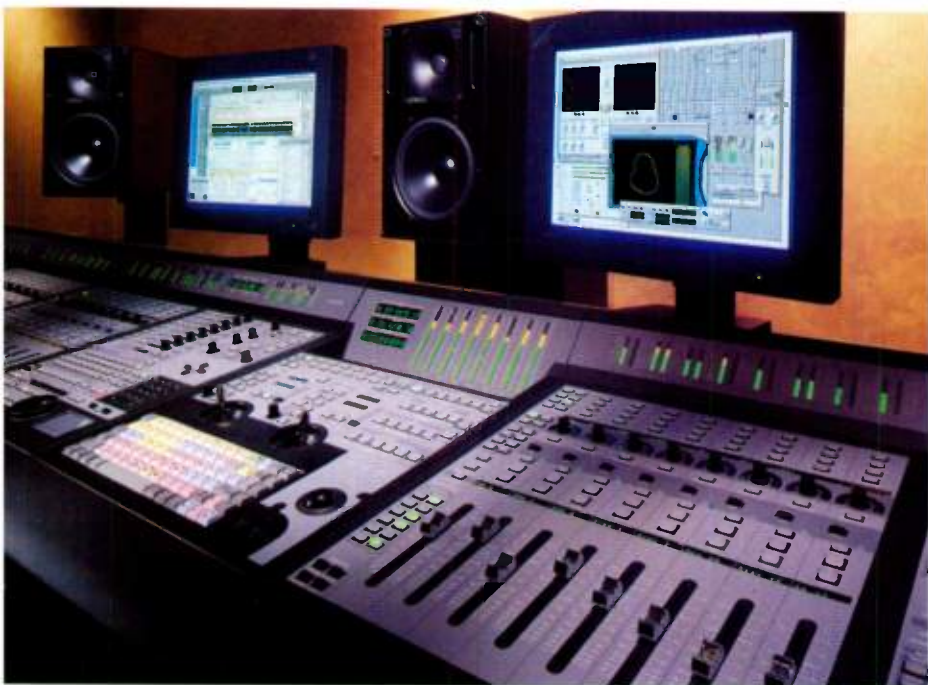
A top-of-the range Pro Tools TDM setup, running processing plug-ins (visible on screen) with an expanded ProControl hardware control surface.
