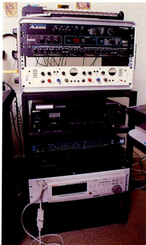
Some of the gear in Dare Mason's studio. From top: Alesis Microverb 3 and Lexicon Alex multi-effects, Alesis 3630 compressor, TL Audio C5021 valve compressor, Sony DAT recorder, MOTU 2408 recording interface and Fostex D160 hard disk recorder.
