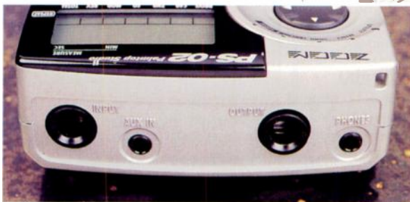
The mono, quarter-inch jack input can accept a range of guitar, synth or mic inputs. Output is via a stereo quarter-inch jack, though a 3.5mm mini-jack output is included for headphone use. A stereo mini-jack Aux In is also provided.
