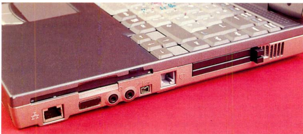
The right-hand side of the laptop features a built-in floppy drive, as well as the two PCMCIA slots, FireWire port, Ethernet port, headphone and mic sockets, and modem connector.
