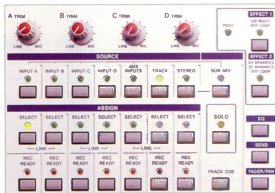
The assignable mixer section of the Tascam 788.
