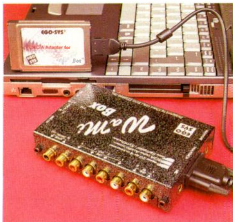
The WaMi Box's audio I/O is handled using gold-plated phono connectors.
