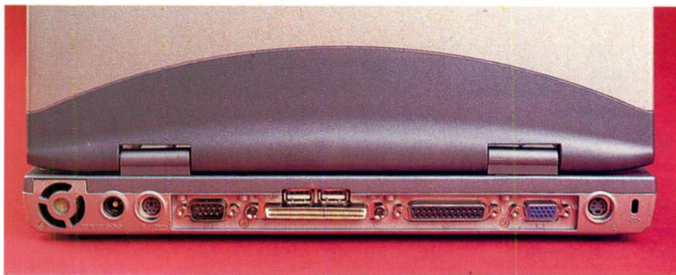
The back panel sports a PS/2 mouse/keyboard port, a serial port, two USB ports, a parallel printer port, outlets for a VGA monitor and S-Video TV display, and a Replicator port allowing you to duplicate the functions of these ports on an external Port Replicator.
