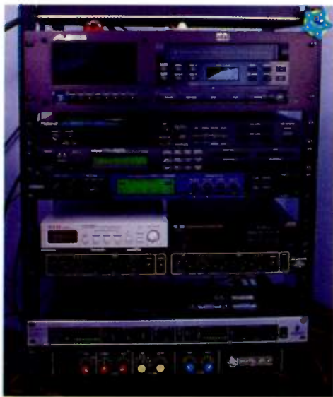
The Alesis ADAT 8-track digital recorder takes pride of place at the head of Raj's main rack.
