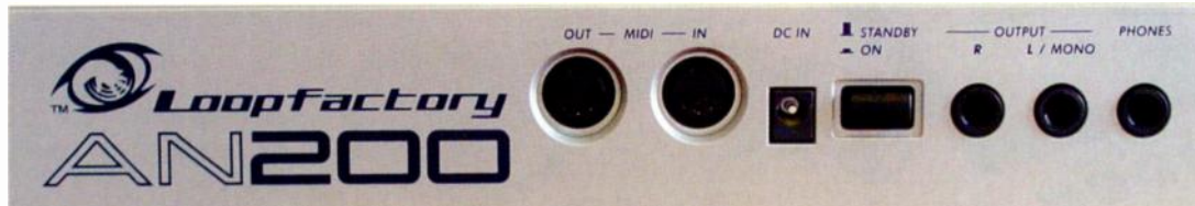
The AN200's rear panel. Note that there are only two MIDI sockets, In and Out, with the Out configurable as a 'soft Thru'.
