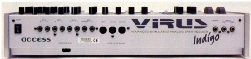
The Virus Indigo's comprehensive I/O facilities: stereo analogue ins for external audio processing via the synth engine, three pairs of analogue audio outputs (four of which can be used to produce a quadrophonic output), MIDI In, Out and Thru, the headphone socket, and pedal inputs.
