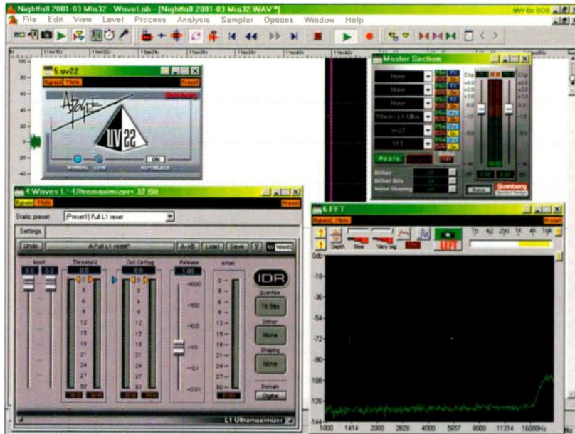
The FFT display, bottom right, shows the high-frequency dither noise added by the popular Apogee UV22 algorithm.
