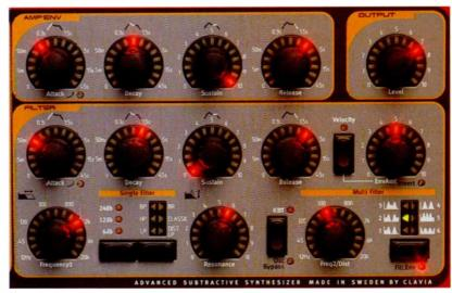
controlling the amount of clip distortion. Finally, there is Distortion Modulation, in which the combined output of the two oscillators is amplitude-modulated by a third, 'hidden' oscillator whose pitch is controlled by the Modulation knob, and the result is routed through a distortion
