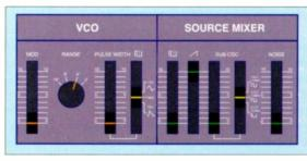
Figure 3: The SH101 oscillator and mixer settings.
