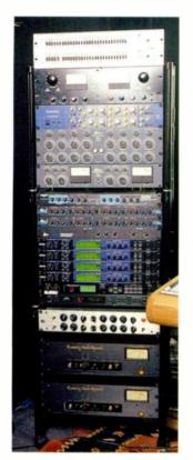
Chris' compressors and other gear (from top): graphic equaliser, Chiswick Reach stereo valve compressor, Focusrite ISA430 input channel, Prism Sound MEA2 EQ and MLA2 stereo compressor, RSP Hush 2000 noise suppressor, Dbx 274 (x2) dynamics processor and 120XP subharmonic synthesizer, Yamaha REV500 (x4), D6000 and SPX990 multi-effects, Summit Audio EQP200B EQ, and Esoteric Audio Research compressors (x2).
