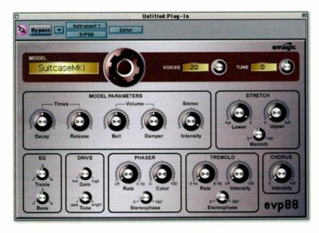
loading user patches, and in addition to the basic piano, there's also a supremely nice Phaser, Tremolo and Chorus section. A couple of smaller dials at the top of the window set the maximum number of voices (up to 88) and permit finetuning, and as the name of the plug-in suggests, it responds to MIDI notes over the full 88-note range.
