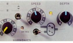
An LFO sawtooth waveform and envelope triggering mode are accessed from a new three-position switch.
