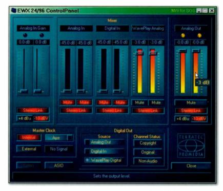
the source signal is when recording from another record or playback device such as a DAT or Minidisc machine. Assuming your mix was correctly recorded onto this device in the first place, you will already have a signal whose peak level is within a few dBs of digital clipping at the nominal level. When transferring this signal to your soundcard you should therefore choose the same nominal sensitivity as your DAT recorder output.
