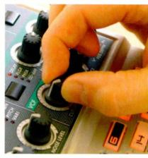
Tweaking the cutoff parameter of the DX200's resonant filter.
