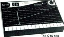
sixteen 60mm sliders. These sliders may be assigned to a variety of MIDI control functions, which are held as one hundred templates (Targets). As the C16 is mainly a preset device you avoid the brain-ache of having to program it yourself, and you can quickly get stuck in to using it creatively. The large number of presets (ninety-eight) means that C16 is ready, out of the box, to do most of the jobs that you are likely to want it to do.
