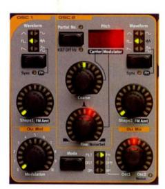
The two oscillators can now be used for FM synthesis in addition to their analogue modelling duties.
