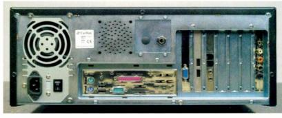
components Carillon had used in their design, and to do this I needed to gain access to the interior of its case. A total of seven screws needed to be removed before the 2mm thick steel cover could be slid rearwards, and of course you would need to unbolt the ACI from a rack to do this. Once
