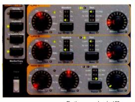
The three comprehensive LFOs offer a variety of waveforms and an impressive range of frequencies and modulation destinations. To the left, the Morph Assign controls govern the allocation of morph functions to controllers such as the mod wheel, keyboard velocity, and aftertouch. The infinite rotary encoder knobs and their LED 'collars', which contribute so much to the visual appeal of the Nord Lead 3, are particularly in evidence here.
