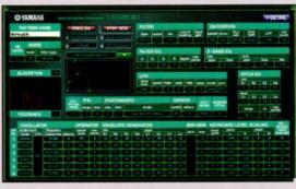
The main Voice Editor window, showing the many parameters that can be edited in depth, particularly the FM algorithm operator parameters on the bottom third of the screen.
