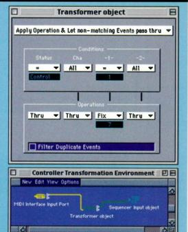
The Environment cabling and Transformer object settings which will convert mod wheel messages to any other MIDI controller number.
