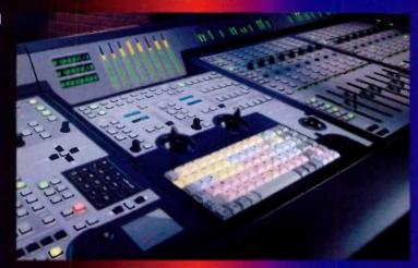
With 16 Focusrite Mic Preamps, 24 motorised Control 24 faders, transport controls, and a master section, Control 24 brings the look and feel of a conventional mixing desk to a Pro Tools workstation.
