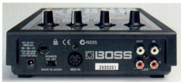
The rear panel, from left to right: the 9V power socket, Kensington security cable slot, Power On/Off switch, the solitary MIDI In, and the Line Out and In phono sockets.
