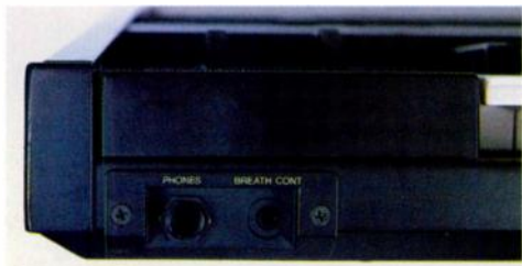
Breath control was an unusual expressive feature offered by the DX7. The breath controller input is found next to the phones socket on the left front edge of the synth.
