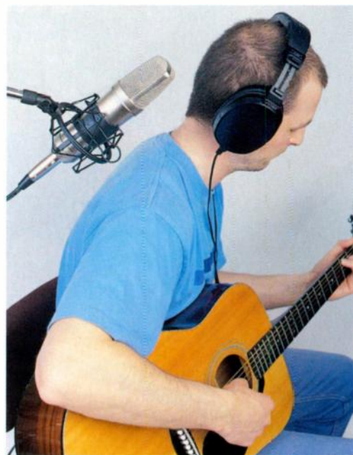
In the right room, this mic placement can produce a sound similar to what the guitarist is used to hearing.
