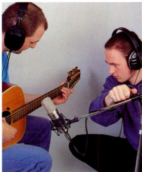
Moving the mic whilst monitoring on headphones is the most effective way to fine-tune the position.
