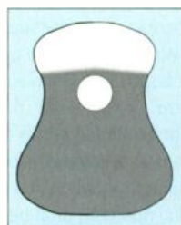
Figure 7(a): The 0,0 mode of a guitar plate.
