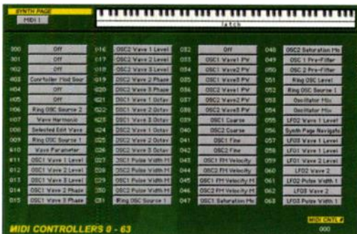
Two of Synthesizer One's eight editing pages are devoted to MIDI control. Over 300 Sz parameters can be controlled, using all 128 possible MIDI Controllers if need be.
