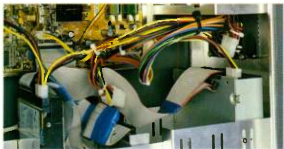
Although rounded IDE cables facilitate a smoother airflow through your PC, flat 80-way cables such as these can give more reliable CD burning performance.
