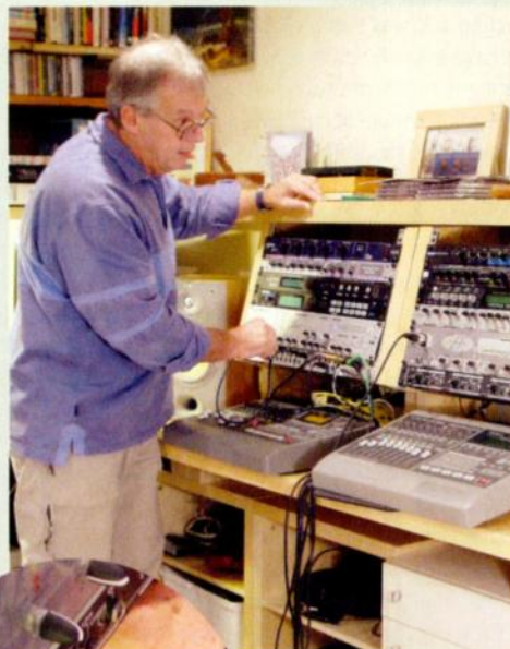
Alan with his two Roland VS recorders. The machines were sync'ed up using MIDI Time Code and MIDI Machine Control, allowing him to record up to ten tracks at a time. To get audio from the slave VS880EX to the master VS880, the S/PDIF output of the slave had to be connected to the S/PDIF input of the master.
