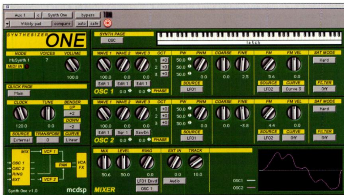
Synthesizer One's editing window, with the Quick edit page on the left above the routing diagram. The main area of the plug-in window shows the Oscillator page: each 'VCO' can blend up to three waveforms, with powerful FM and ring-mod possibilities.
