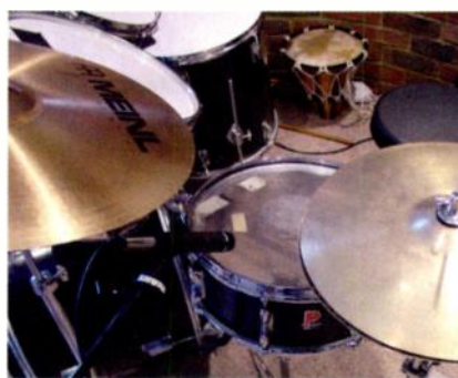
An SM57 was positioned looking over the top lip of the snare, pointing towards the centre of the drum and away from the toms.
