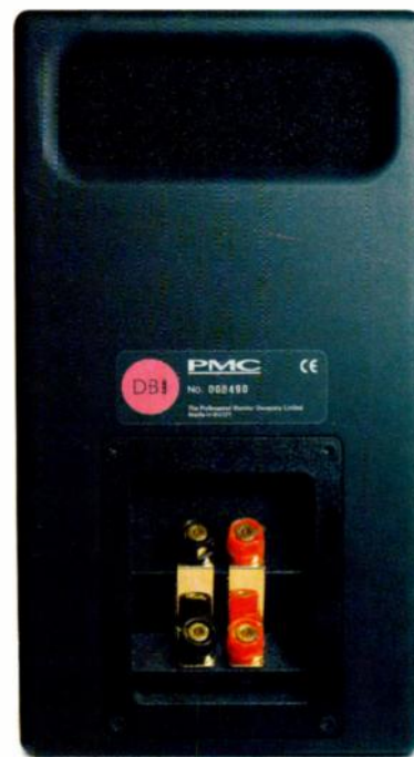
The transmission line vents at the top of the rear panel, so placement of the speaker near walls should be avoided. Four binding posts allow bi-wiring and bi-amping.
