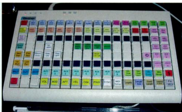
Hans Zimmer's custom keypad: notice the yellow keys along the bottom for switching Controller Lanes and the light-purple keys at the right for triggering Logical presets. The two rows of black keys are there to make the keypad easier to navigate.
