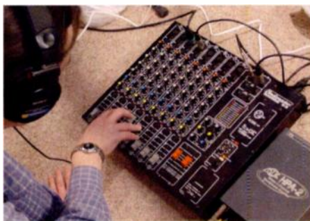
An old Studiomaster console was used to supply phantom power to the two Rode NT1s overhead mics.
