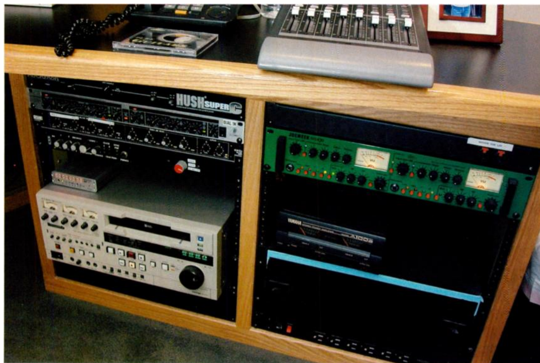
The right-hand rack in the composition area, including Rocktron Hush noise suppressor, Behringer Composer compressor, Rane preamp/mixer, professional VHS machine, Joemeek TwinQcs voice channel and Yamaha A100 power amp.
