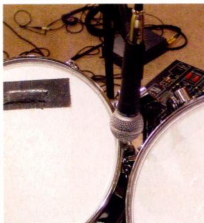
An SM58 was used as a close mic for the toms, and was pointed downwards to minimise cymbal spill.
