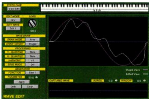
As well as providing a good range of standard waveforms, Synthesizer One offers the option to capture additional waves from incoming audio or draw your own with the mouse. The results can be used both by VCOs and LFOs.
