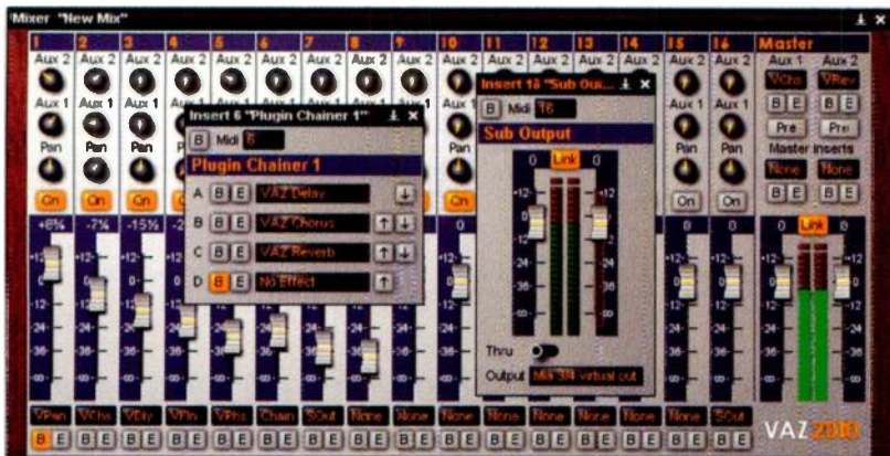
The 16:2 mixer provides aux and insert effect slots, accepts both VST and DX plug-ins, and is supplied with eight bundled plug-ins of its own.
