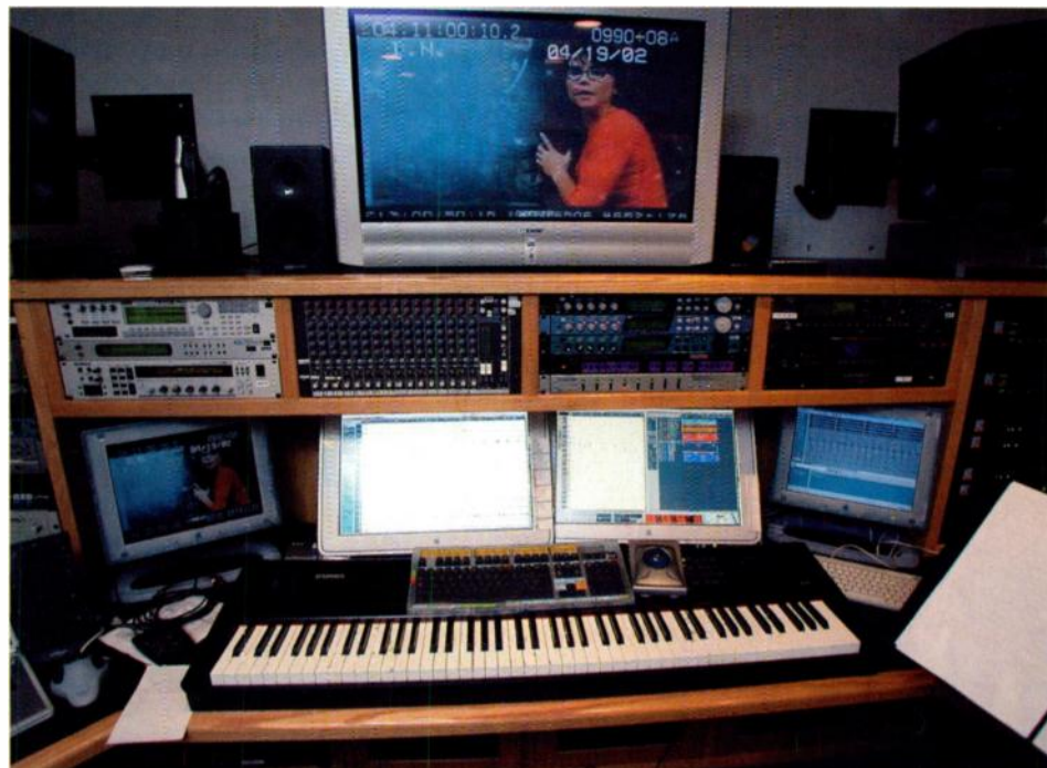
David Newman's main workstation in the composition room, with no fewer than three computer screens and two video displays. Visible in the rack are (from left), Korg Triton Rack and TR-Rack modules, Yamaha CS6R module, Mackie line mixer, Emu Proteus 2000, Audity 2000 and Planet Earth modules, Roland XV5080 module and VP9000 processor.
