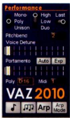
The label 'D:16' in the polyphony display signifies that 16 voices are under the control of the new dynamic voice-allocation mode.
