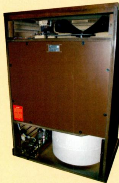
Inside the 122XB. The treble horns can be seen at the top of the unit, while the rotating polyurethane drum which shapes the sound of the bass speaker is visible at the bottom.
