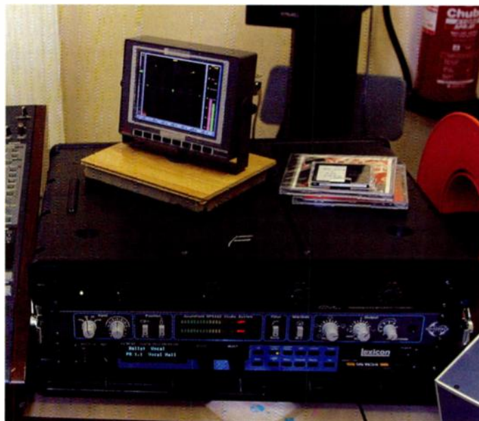
The GML mic preamp at the top of the rack was used for the vocal mics, whereas the processor below it was used to control and decode the Soundfield mic above the drum kit. At the bottom of the rack is a Lexicon PCM90 reverb processor which was used for vocal reverb. A DK Audio MSD600M meter sits atop the rack.
