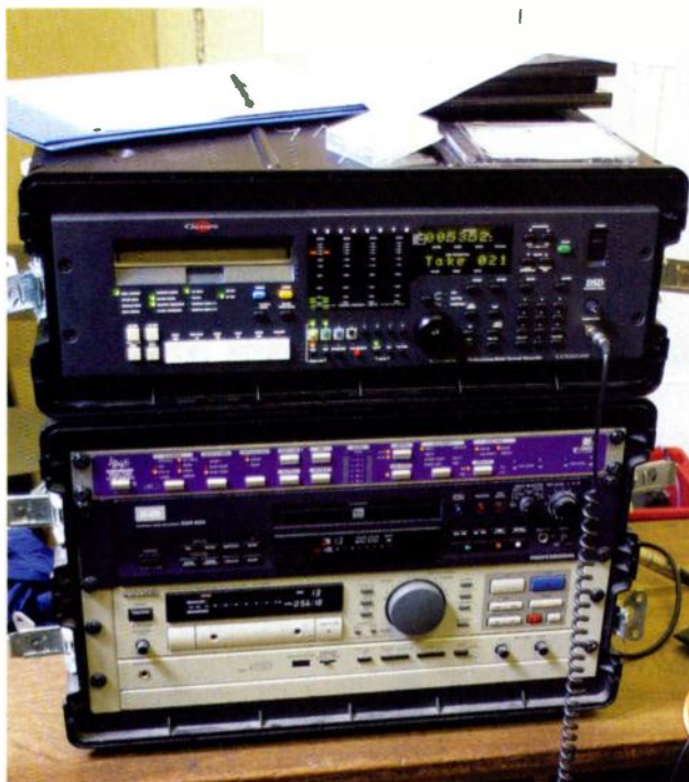
A Genex GX8500 was used as the master recorder, with a DAT machine providing backup. The Apogee PSX100 converter provided digital routing to the DAT and CD-R machines, as well as acting as an A-D for playback.
