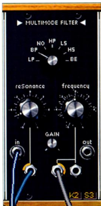
The 12dB-per-octave multi-mode filter. Note the yellow 'value' collars around the modulation inputs. The digital display in the corner shows the filter is routed to key follow 2, and sequencer row 3.
