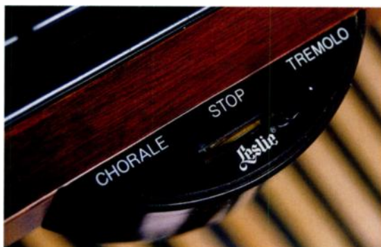
The Leslie controls on the B3 itself. Care needs to be taken when using these in conjunction with the Leslie speed switch on the expression pedal, though, as the switch here can get out of sync with it.
