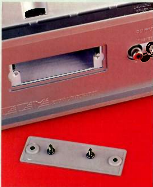
An expansion slot at the rear of the unit accepts an optional USB interface board, allowing you to hook the MRS802 to your computer for backup and audio CD-writing purposes.
