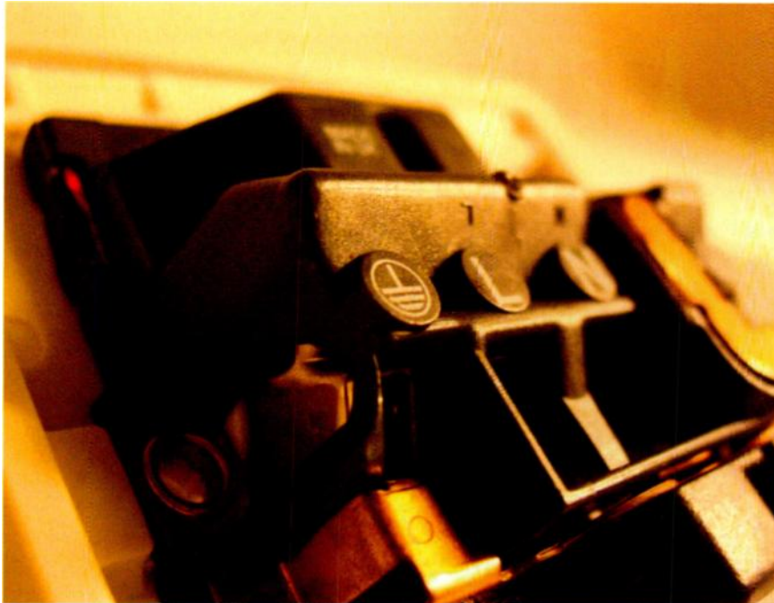
Though essential for electrical safety, the mains earth connection is also a common source of RF contamination.
