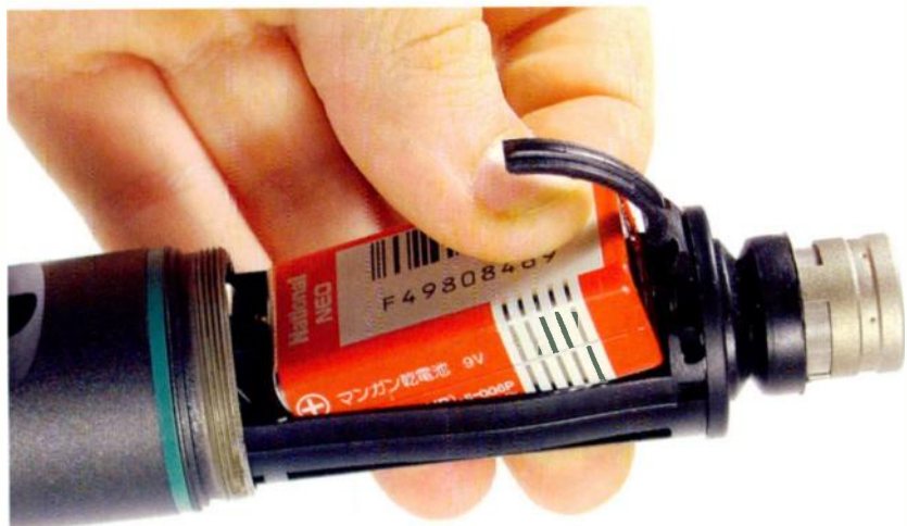
The AKG C1000 back-electret mic can be powered either from a normal phantom supply, or from a 9V battery fitted inside the mic casing. The option of battery power could be very useful if your mixer or recording channel has no phantom powering option.
