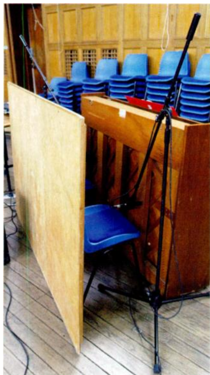
A piece of stage scenery was used as an impromptu screen to increase separation for the piano mics. However, this made the sound quite boxy, so some corrective EQ was required at the console.
