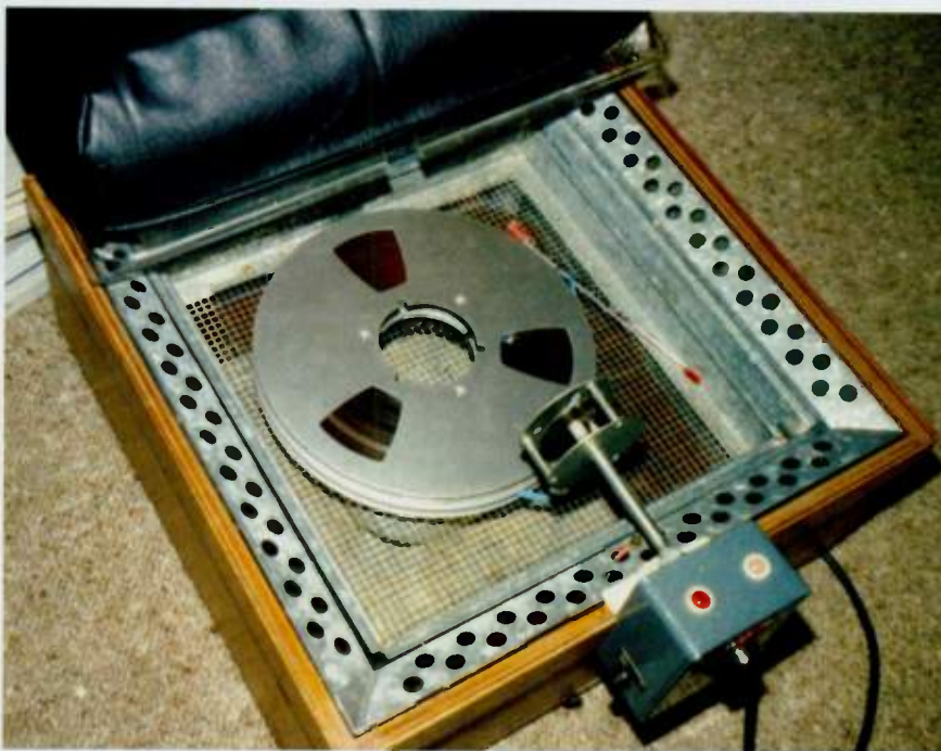
Paul White's Ampex reel-to-reel tapes, ready for baking in a chicken-egg incubator. Delicious!
