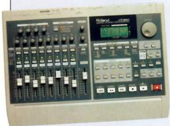
The venerable Roland VS880 multitracker can connect to external drives via SCSI.
