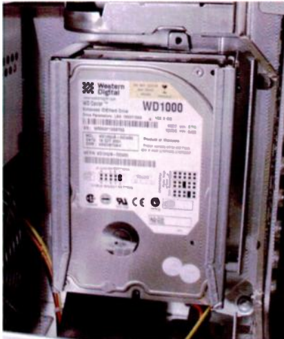
Two Western Digital WD1000B drives in position on the test Mac's ATA100 buss.
