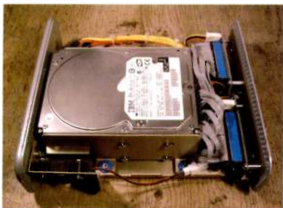
The Mediabank MTR open to the world with test drives newly installed. It's a very snug fit!
