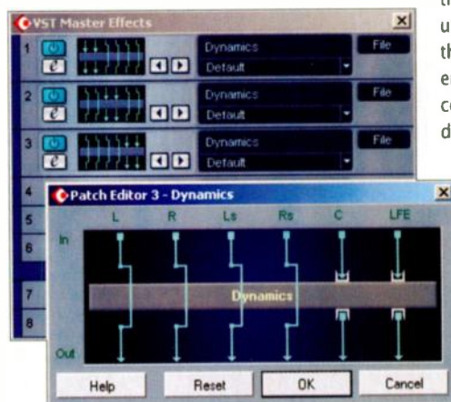
Figure 6: In a surround project, two-channel effects plug-ins can be applied to individual pairs of outputs via the VST Master Effects window.
