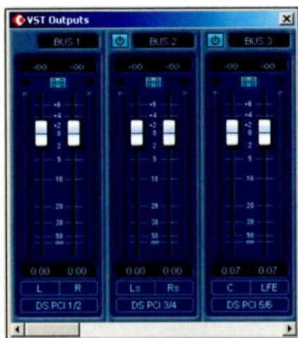
Figure 2: Hardware outputs are assigned in the VST Outputs window.
