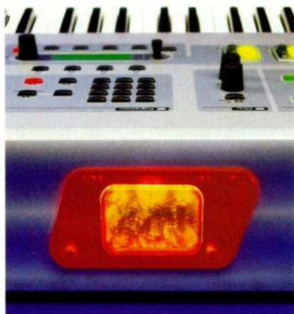
As the Neuron's connections are all located on its side, the rear panel contains only the stylish Hartmann logo, which doubles as the On switch.
