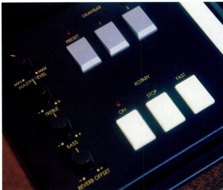
Simple EQ controls situated on the lower keyboard add the potential for quick and easy treble and bass tone shaping.
