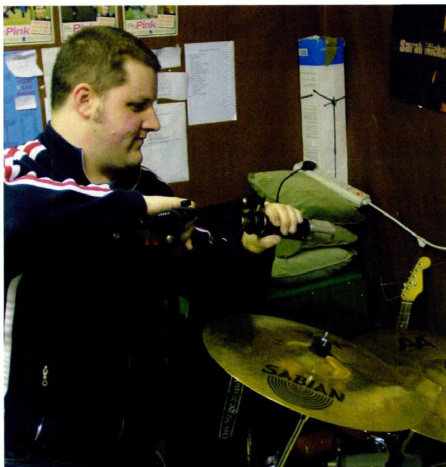
In order to widen the stereo image of the kit, the single Rode NT1 which Ian Anderson had been using as an overhead mic was replaced with a matched stereo pair of Groove Tubes GT55s. Here you can see Ian positioning one of these mics to get the best balance of cymbals.
