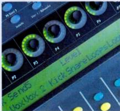
Your hardware and software may not correctly interpret the MIDI output from endless rotary knobs, like those on the Steinberg Houston.
