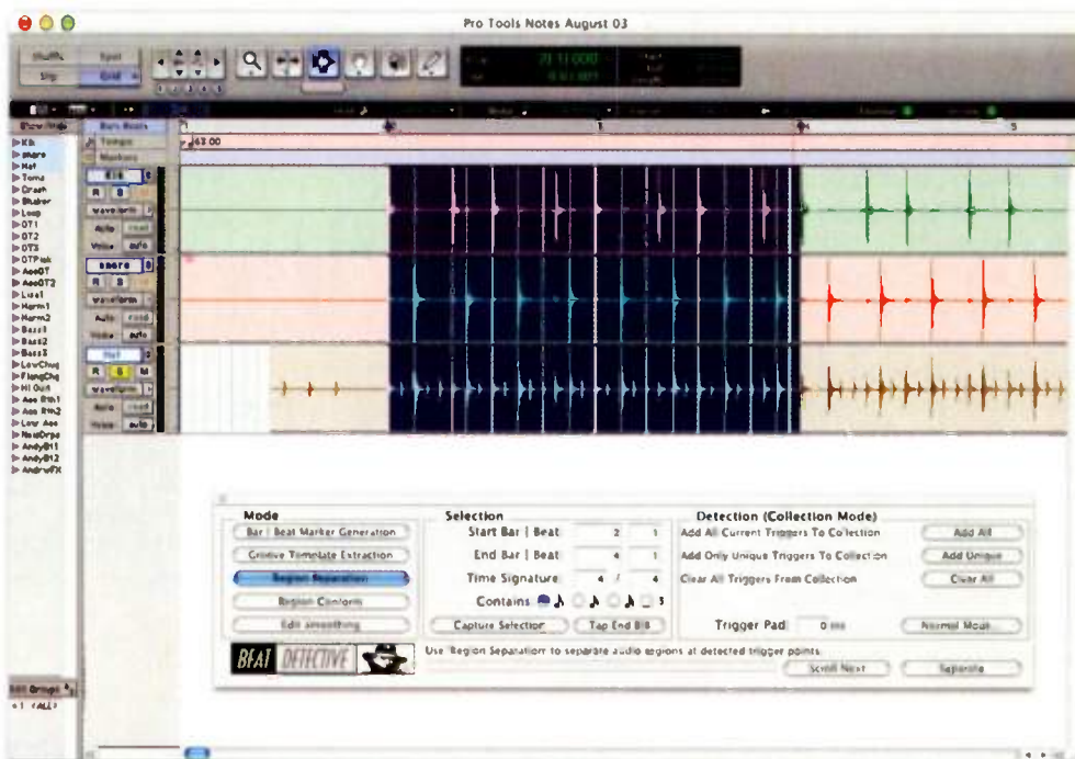
Collection mode allows you to amalgamate the transient information from several multitracked parts.
