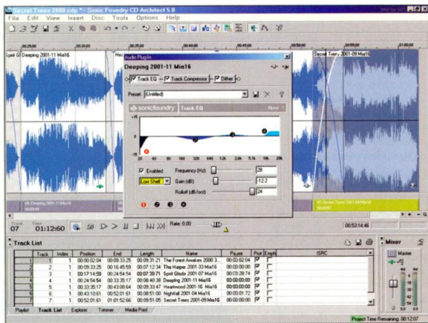
Dedicated pre-mastering and CD-burning applications like CD Architect 5.0 let you apply a different complex chain of plug-ins to each successive track, with the plug-ins only consuming CPU while that track is playing.
