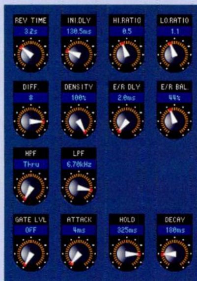
Here you can see the range of editable parameters available for one of the 01V96's internal reverb algorithms, as presented in Studio Manager .
