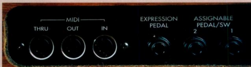
At the back you'll find the MIDI, Expression pedal and two additional assignable pedal sockets.
