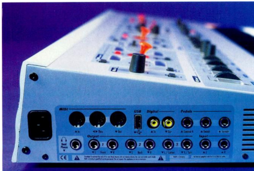
Everything on the side; even mains power is provided via an IEC socket on the side of the Neuron. The all-important USB jack here is where the Modelmaker software is connected (via a suitable USB-to-Ethernet adaptor). Sadly, the two audio inputs are not yet functional.
