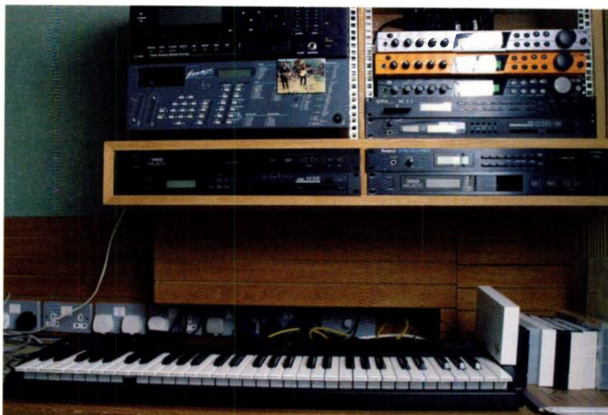
The only sampler in Tot's studio is his ancient Emu Emax rackmount, which is no longer used. Other MIDI sound sources include Emu Proteus 2000, XL1 and Virtuoso 2000 modules, Kurzweil K2000R, Roland D110, Kawai K1R, Korg O3R/W and M3R modules, and a Korg X5D used as a controller keyboard.
