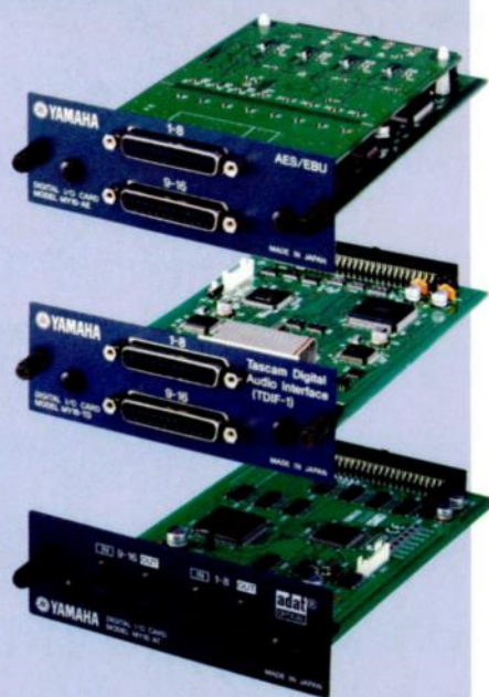
The MY16AE, MY16TD and MY16AD 16-channel digital interfacing cards let you maximise the 01V96's input capacity.
