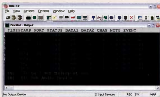
Direct USB-connected MIDI signals between a musical keyboard and your PC may arrive slightly earlier than via a separate USB MIDI interface, as you can see here, with up to 3ms difference between the two routes.
