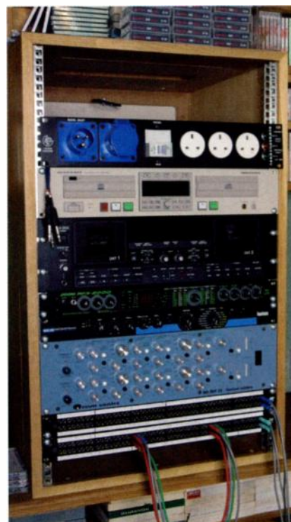
Some of the outboard in Tot's MIDI suite: from top, Marantz CD recorder, dual DAT deck, Zoom RFX2000 and Lexicon MPX100 effects, Oram HD-DEF 35 EQ.
