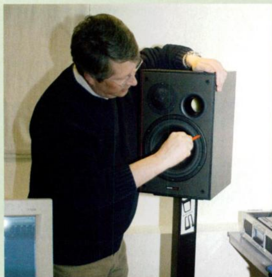
Hugh's first step when attempting to eliminate a rattle in one of the BM5 speakers was to secure some loose fixing screws on the bass driver. When this didn't solve the problem, Paul used a Roland JP8000 to provide a consistent signal, allowing Hugh to troubleshoot further.
