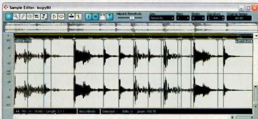
The Hitpoints mode in Cubase SX is designed to detect and mark individual hits, making beat-slicing easier.
