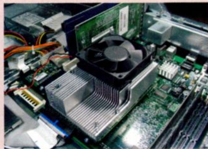
Then the new processor, with its heatsink and fan, is screwed in its place.
