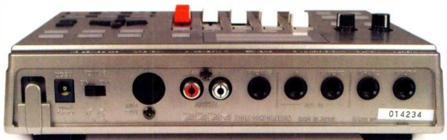
Two tracks can be recorded simultaneously, and an additional pair of input jacks allows you to play along to a drum machine or sequencer.
