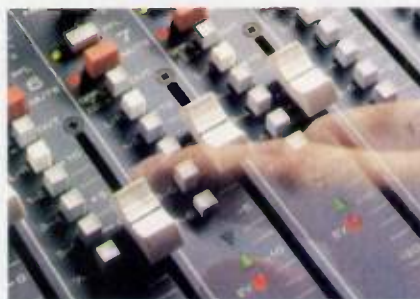
The Solo, PFL and AFL options on well-specified mixers allow the engineer to hear what's happening at different points in the channel's signal path.
