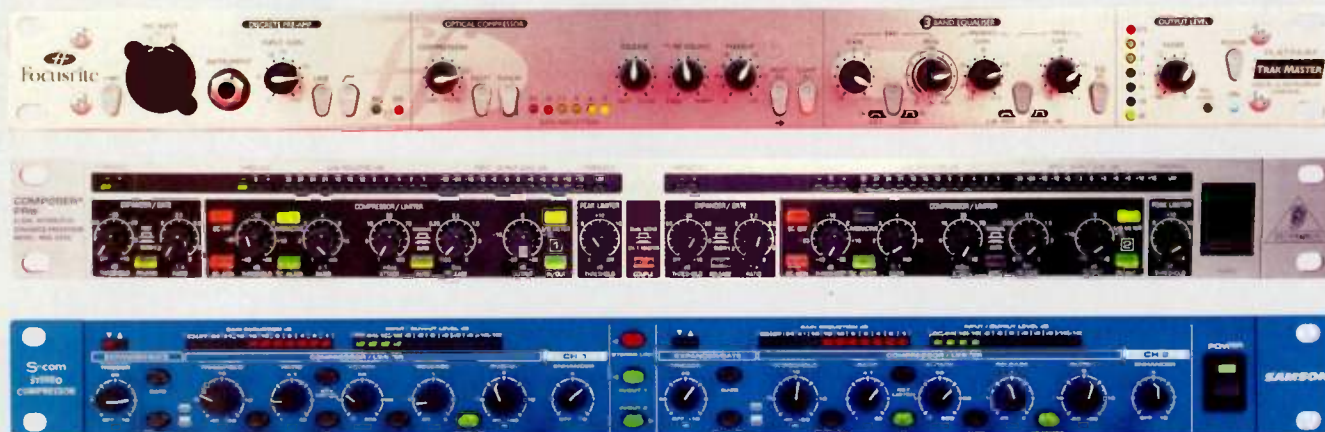
The Focusrite Trak Master and Behringer Composer Pro are two affordable compressors which use optical gain control elements. The Samson S•Com, however, uses a VCA.
