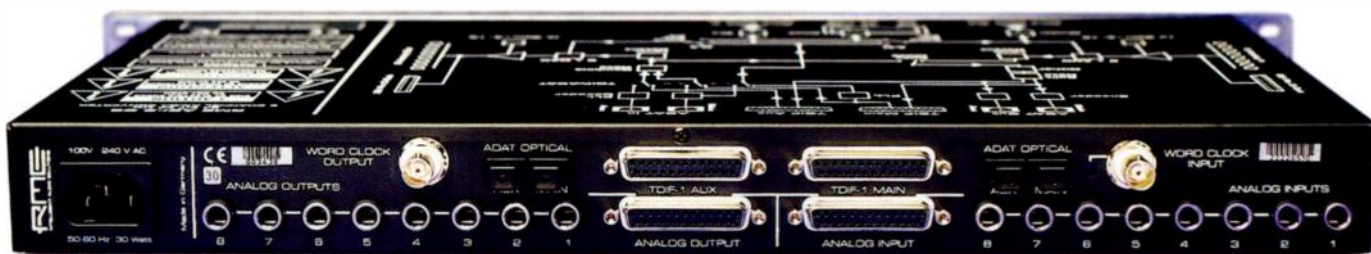
If you weren't certain from looking at the front panel, the back panel makes it clear just how versatile the AD18 DS is, with all eight outputs available on the left (on jacks, analogue 25-pin 'D'-sub connector, Main and Aux ADAT optical connectors), all the inputs available on the right in the same formats, and the bi-directional TDIF-format digital Main and Aux connectors on 25-pin 'D'-sub connectors in the centre. A word-clock in and out (the input with recessed 75Ω termination button) complete the picture.
