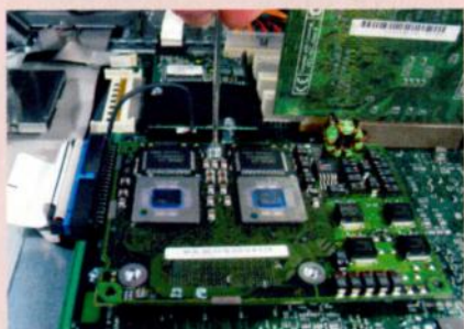
Installing the upgrade in the 450MHz G4 Tower was easy. First, the old processor is unscrewed...
