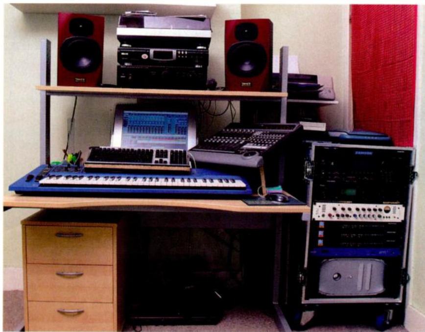
Steve and Dave do most of their programming and mixing in Steve's London flat, but often need to take their setup to studios to record, so it is kept in a mobile rack. The core of the system is a G4 Mac with a Pro Tools Mix Cube system running Logic as a front end.
