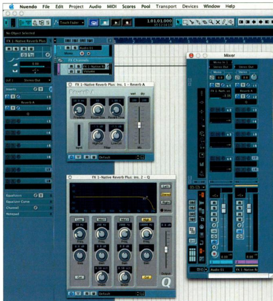
Send effects in Nuendo 2 are handled by dedicated FX Channels on the Mixer and Project windows, enabling you to stack up to eight effects per send effect buss.
