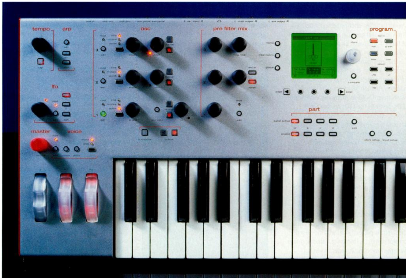
The Ion's control panel is laid out from left to right to reflect its signal path, with the controls for its three oscillators on the left, followed by a pre-filter mixer. Performance controls, such as the three lit wheels and the buttons governing portamento and the arpeggiator, are situated at the edge of the control panel and fall easily under your left hand.
