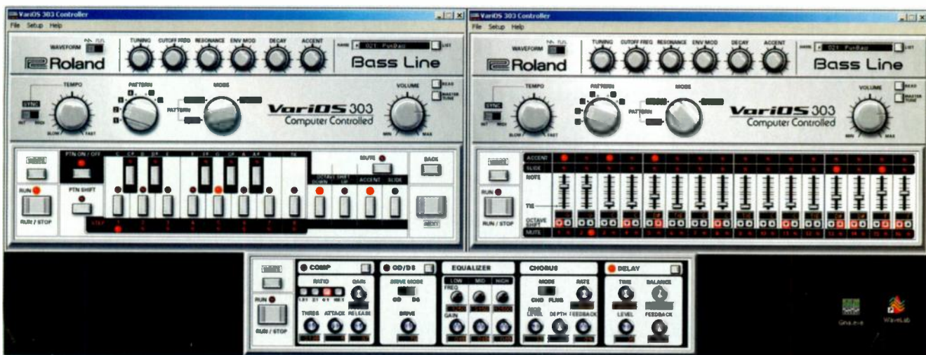
The VariOS 's TB303 emulation, VariOS 303 . The screen on the left here shows the step-sequencer mode, while in the other, each individual step is editable on its own slider (try doing that on a real TB303). The built-in effects can be seen in their own window at the bottom of the screen.
