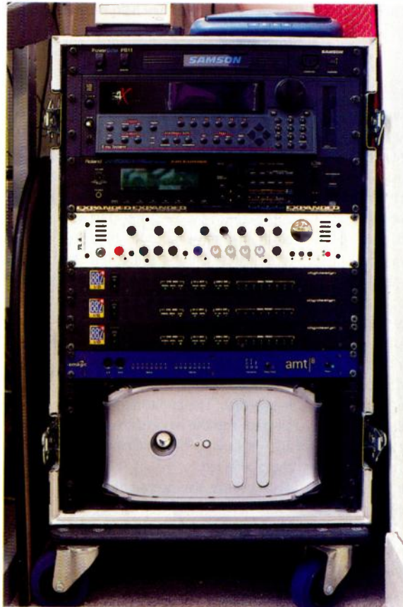
The duo's mobile rack contains (from top) Emu E4X sampler, Roland JV2080 sound module, TLA Ivory voice channel, Digidesign 882 I/O interfaces (x3), Emagic AMT8 MIDI interface and Apple G4 Mac computer.
