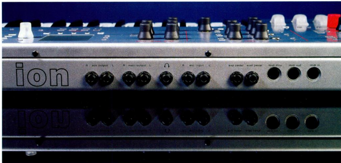
The Ion's rear panel sports two stereo outputs, a headphone jack, a stereo input, and sustain and expression pedal connections. There are also the usual MIDI In, Out, and Thru sockets.
