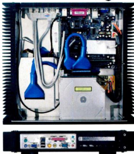
The new Hush PC: it has no cooling fans (hence all the fins) and is virtually silent. A recording musician's dream?
