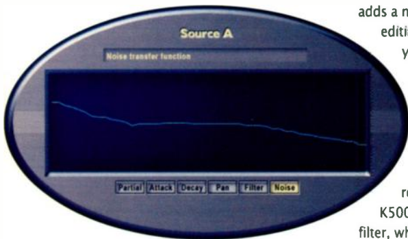
Cube's oscillators generate noise by modulating the partials used in the sound. This can then be introduced into the oscillator's output by drawing a noise transfer function across the frequency spectrum.
