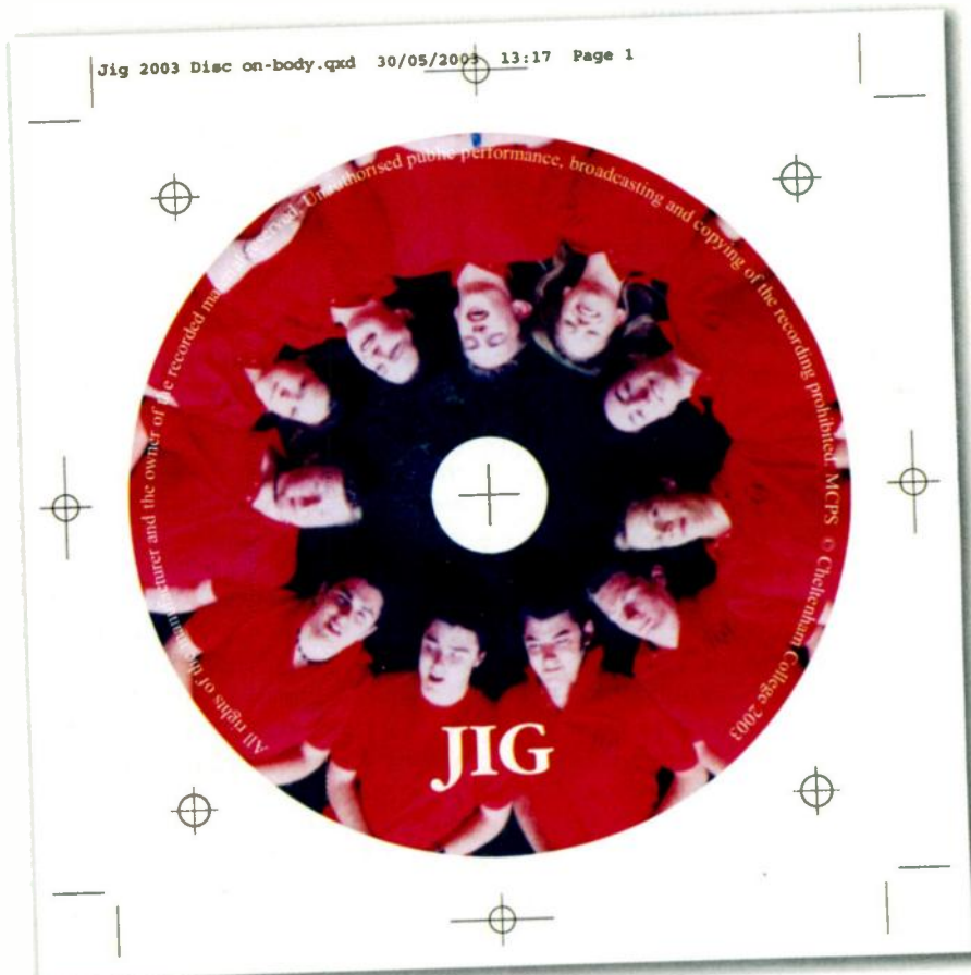
The artwork proof for the on-body CD printing — the size of the hole at the centre of the image is critical, and each pressing plant will have its own tolerances depending on the printing technology used.
