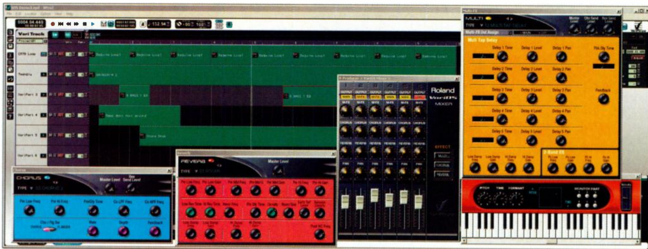
The VariOS's default V-Producer software. The Vari Track window (top left) closely resembles a piano-roll editor in a sequencer. On the right is the VariOS Mixer, and several effects are visible (chorus, reverb, and multi-effects), as well as the on-screen keyboard, which displays input MIDI note data.
