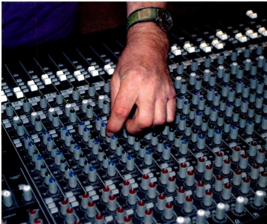
Alistair had been using fairly extreme EQ settings for his bass sounds on his Mackie console — the low-frequency shelf was cranked all the way up, giving 15dB of boost! Paul flattened the bass channel's EQ and resolved to optimise the sound in other ways.
