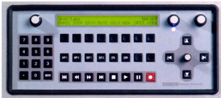
The master control panel, with its alpha stick (bottom right). As is evident in this and the picture on the previous page, front-panel labelling is minimal, because the physical controls can be assigned to so many potential tasks. This is fair enough, but maybe some scribble strips or overlays would have been nice to provide instant reminders of how you currently have the controls set up.
