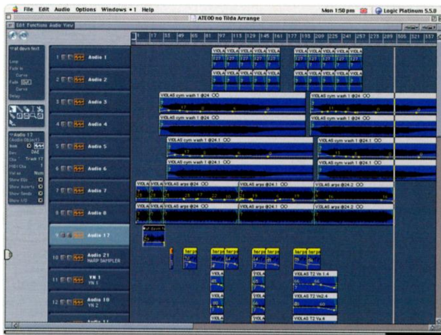
The mix for 'Shadow Journal': the string recordings made to analogue tape at Eastcote are imported into Pro Tools (with Logic as a front end) for editing and combined with the other elements of the track, such as the electronica and spoken-word recordings.
