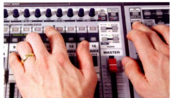
Holding the Automix button and pressing Ch Edit is useful for quickly setting the Automix status of individual mixer channels. You can also use this technique to 'punch in' on recorded automation, but in practice the VS2480 responds a little too sluggishly when you try to do this.
