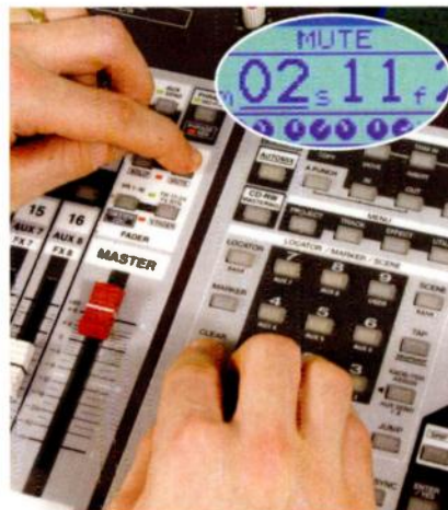
It's easy to leave a track muted without realising, as you only get a small alert message at the top of the LCD. If you see the alert flashing at you, then hold Clear and press Mute to unmute all channels.
