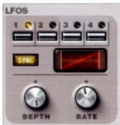
The four LFOs share one set of controls, with the one to edit chosen by the four switches at the top.
