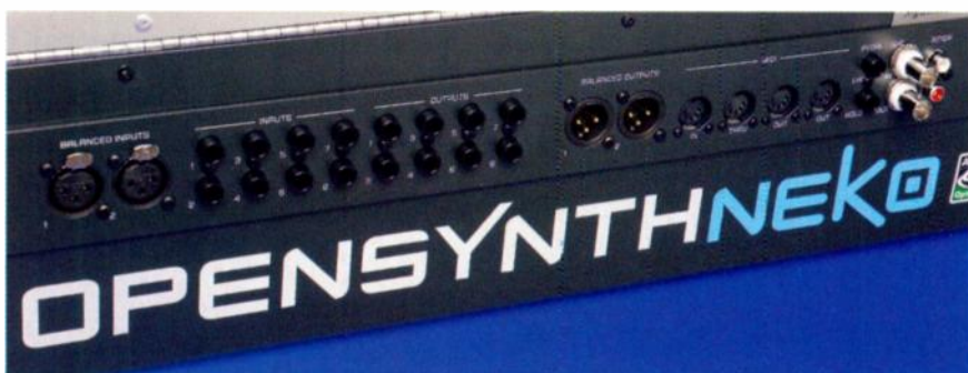
I/O is comprehensive, thanks to Open Labs employing an M Audio 1010LT as the Neko's output stage; there are eight jack ins and outs, plus a further two balanced inputs and two outputs on XLRs. Stereo digital I/O is provided on S/PDIF, and there are four MIDI sockets (the usual three plus an extra MIDI Out), plus connectors for word clock and expression pedals.
