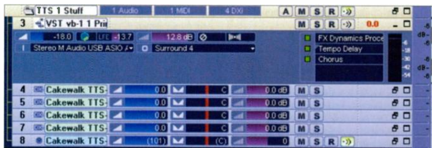
A closer look at Sonar 4 's new track folders option. The new TTSs multitimbral sound module is grouped with a number of individual MIDI tracks that are playing it.
