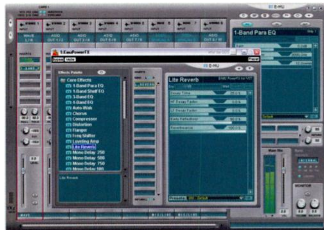
Here you can see the new Emu Power FX window superimposed on the Patchmix DSP utility, both kitted out in an optional third-party tXz 'skin'.
