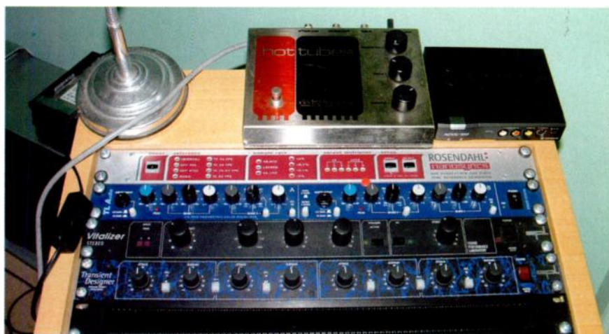
More of Richter's gear (from top): his favourite Electro-harmonix Hot Tubes pedal, Rosendahl Nanosyncs master clock, TLA Indigo stereo EQ, SPL Vitalizer enhancer and Transient Designer.
