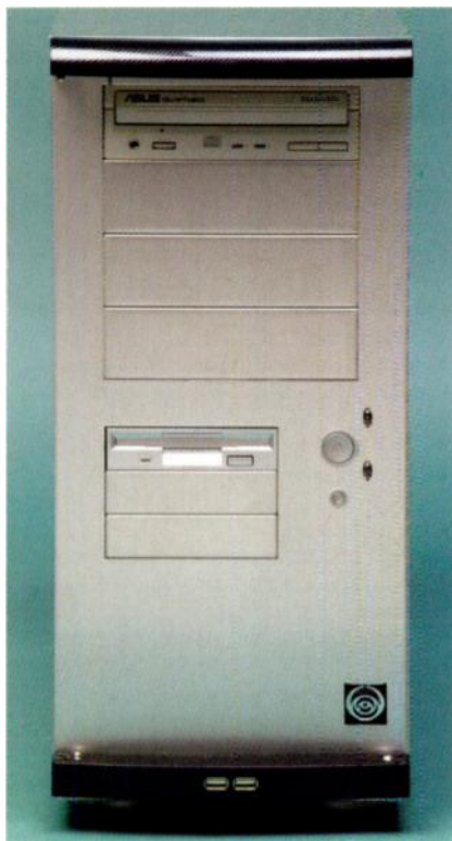
With the main air intake at the bottom of the case, the front panel is both clean and quiet.
