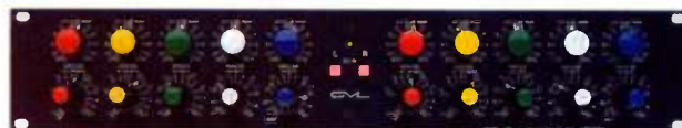
Massenburg 8200 parametric equalizer - reference standard 5 band fully parametric EQ - the most natural of equalizers.
