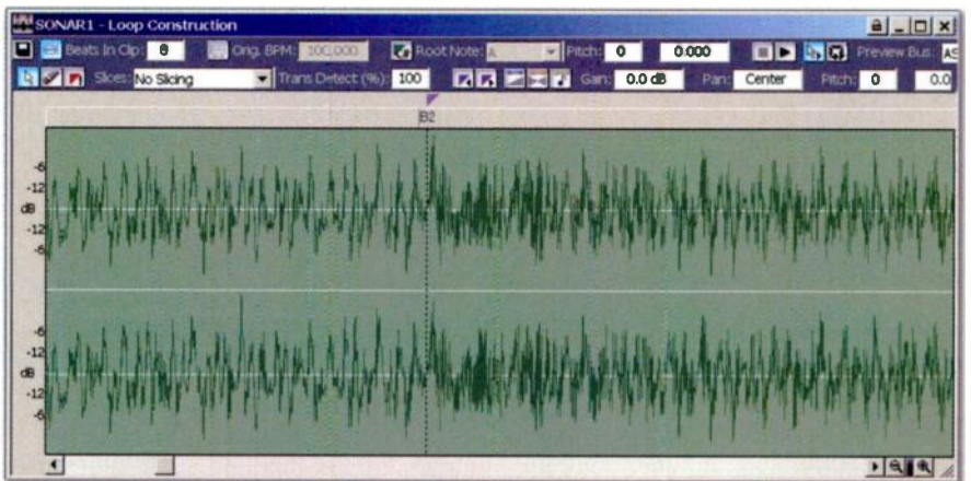
The transient at beat two is difficult to see unless you zoom right in. When you locate it, add another slice marker.
