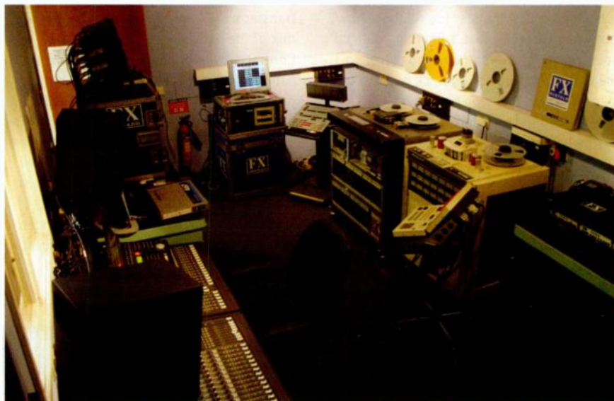
Like all the studios at the Copyroom, Room 1 has a permanently installed Pro Tools system, but at the time of our visit, there was also an old Mitsubishi X850 digital 32-track (in the far right corner), an Otari MTR90 analogue multitracker (the large white recorder to the right of the Mitsubishi), and an IZ Radar (in the middle at the back). Some of this gear is from FX Rentals' stock, wheeled in for as long as it's needed, and then replaced.
