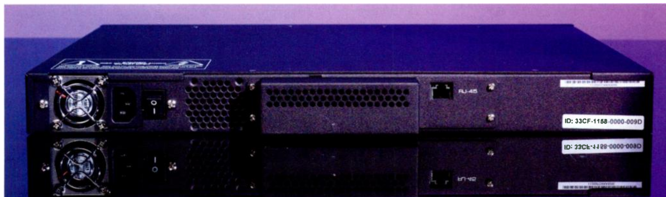
Although the APA 32 is based around a standard ATX PC motherboard, the only connection presented on the back panel is an RJ45 Ethernet port.
