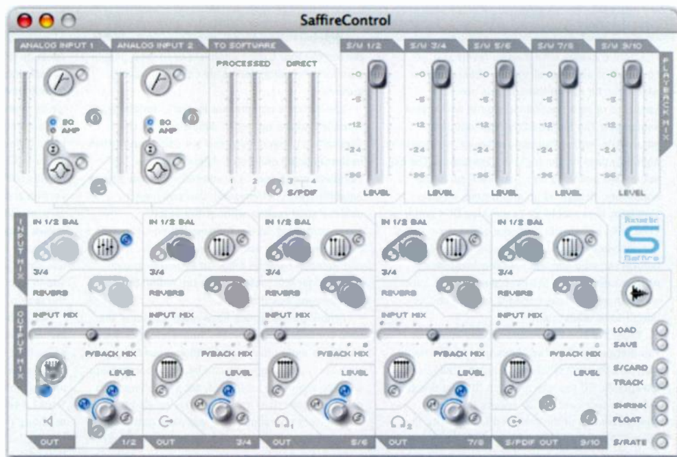
The Saffire Control utility allows you to submit the outputs from your recording application for monitoring, and to set up the plug-ins running on the Saffire's DSP.
