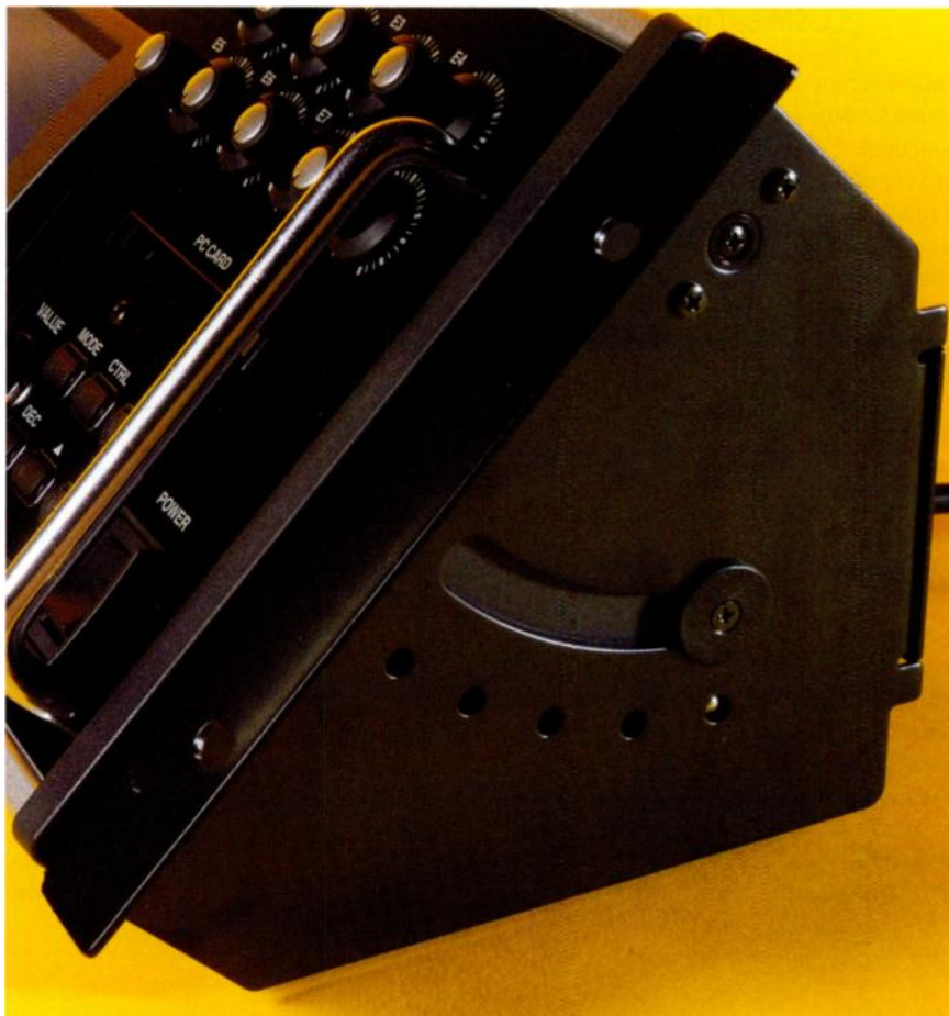
Loosening the large bolt (and its companion at the other end of the V-Synth XT) allows you to slide the rack ears so that you can mount the XT flush or angled in your rack — a nice touch.
