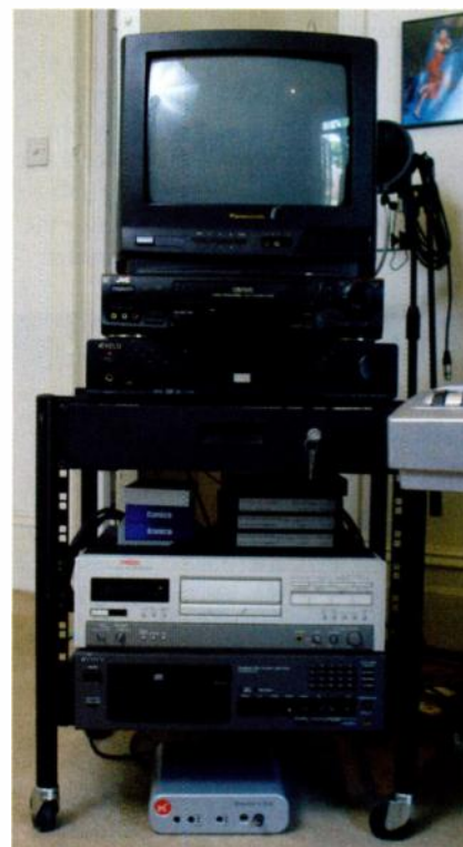
The Miglia Director's Cut conversion box is used to integrate VHS video with Nainita's computer recording system.
