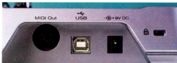
The back-panel view, featuring simply MIDI Out and USB sockets and a 9V power input.
