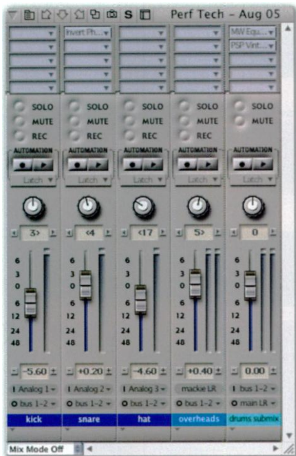
Routing the output of several tracks via a buss or buss pair to an aux track allows them all to share the plug-ins on the aux track. Here several drum tracks are being treated by an EQ and limiter on the Aux (the track at far right)
