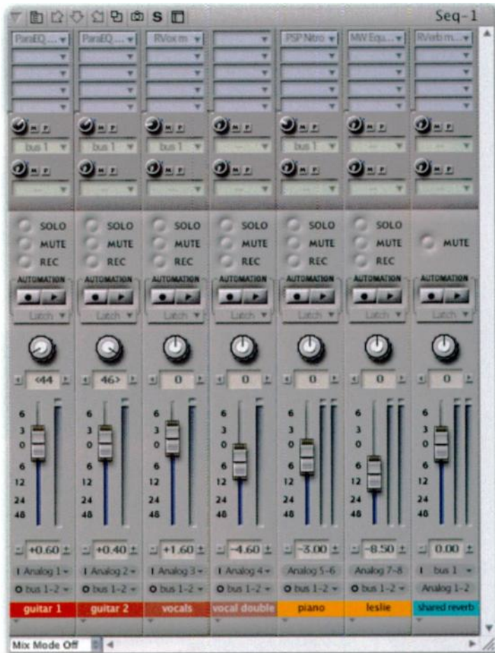
Traditional 'send and return' effects architectures, whereby a single effects processor treat several tracks simultaneously, are easy to set up in DP, and are very processor-efficient. Here the aux track (at far right) is being fed audio via the sends of the audio tracks to the left.
