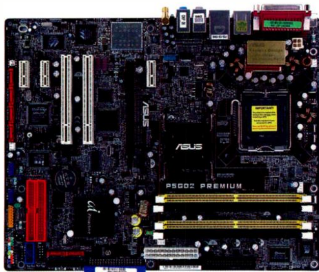
Current PCI Express motherboards, such as the Asus P5GD2 shown here, provide three PCI Express x1 slots, one PCI Express x16 and two legacy PCI slots, but in a year's time PCI support might be dropped altogether from new designs.
