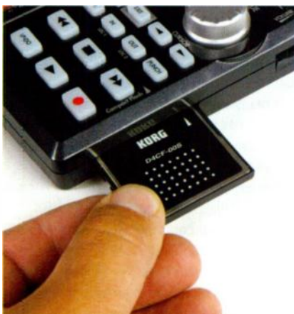
The D4 records directly to an internal Compact Flash card, and capacities of up to 2GB can be used.
