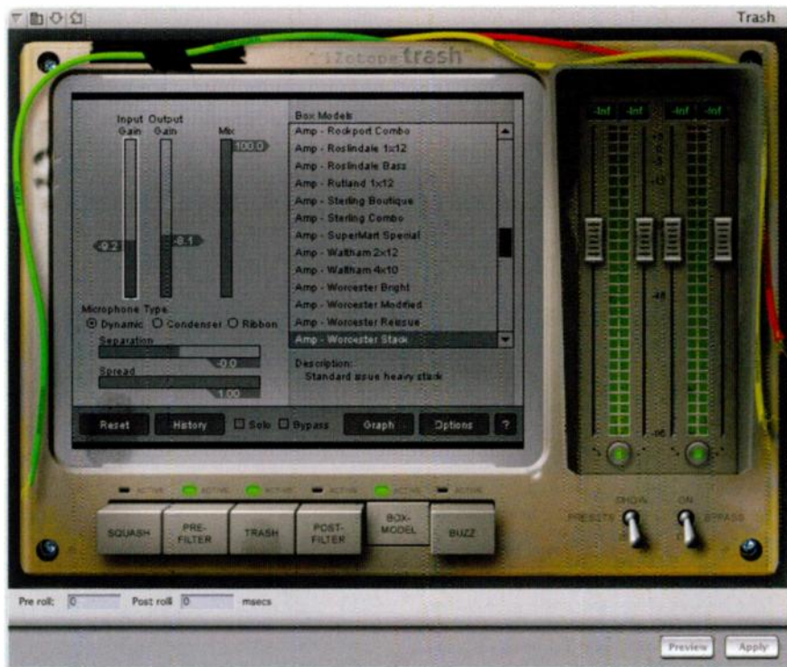
If you know the effect you want, you can apply plug-ins off-line by selecting the audio you want to treat, then choosing a plug-in from the Audio Plug-Ins sub-menu of the Audio menu. With this method, heavyweight plug-ins like iZotope's Trash , shown here, effectively use no processor power at all in your mix.
