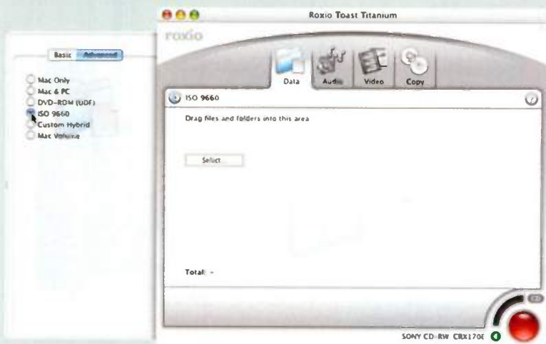
Here you can see the options in Roxio's Toast which allow you to set the format of CDs you burn. ISO9660 is the most widely compatible format, so this is a good choice when you create CD-ROMs for sending final mix files for mastering.
