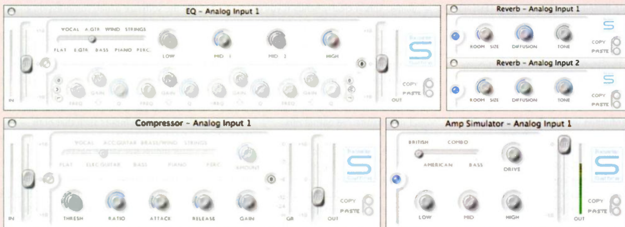
All of the Saffire's DSP effects are also included in VST and Audio Units formats, allowing you to run the same algorithms on your host machine.
