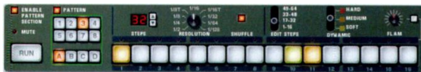
Create patterns by clicking the 16 pad buttons that run along the bottom of Redrum .
