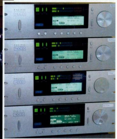
Part of Professor Johnson's bespoke recording rig: four Pacific Microsonics A-D converters, a snip at a mere 30 thousand dollars apiece.
