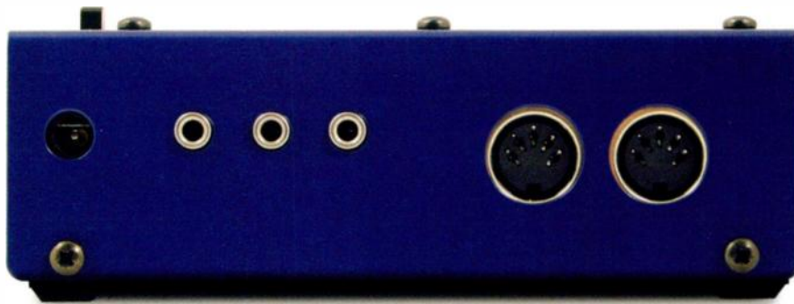
The rear panel may look extraordinarily simple, but there's more to the three plain-looking jack sockets than meets the eye — they're capable of outputting control voltages in a bewildering variety of formats. Even the MIDI Thru can carry Sync 24 or Aux signals as well as MIDI.
