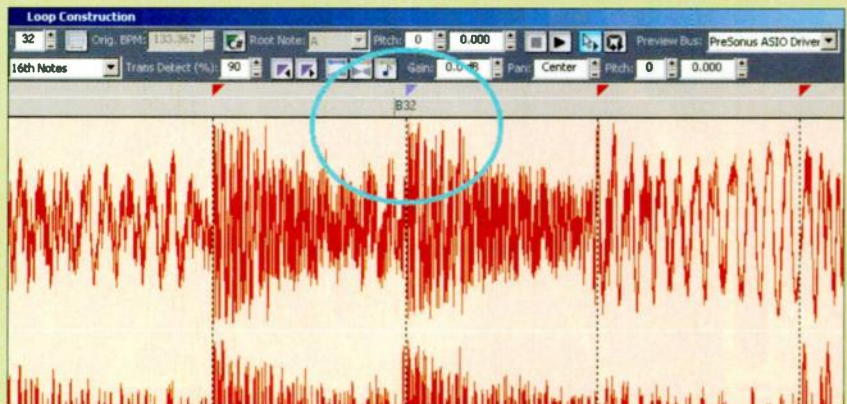
This drum loop was played by a real drummer, so the timing isn't perfect. Sonar originally put markers on every 16th note; but the one circled in blue was moved slightly late compared to the beat in order to fall exactly on the note transient, thus producing the best possible Acidisation .
