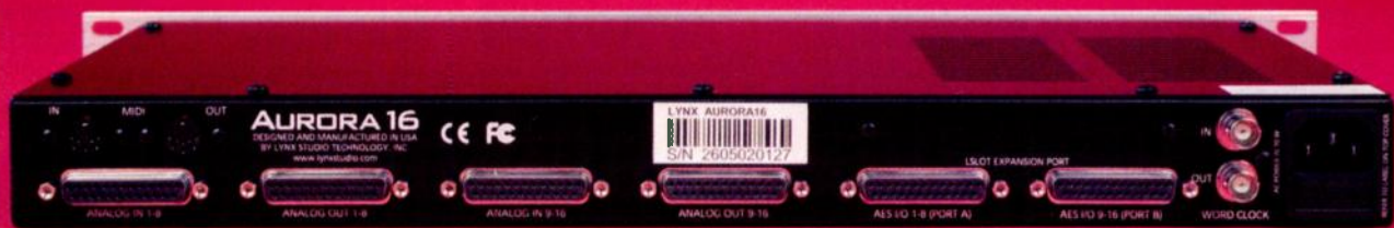
The Aurora connects to the outside world using a bank of D-Sub connectors.
