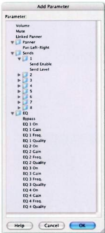
The parameter windows for audio tracks show which parameters can be automated. If any insert plug-ins were used on a given track, the parameters for these plug-ins would show up in this window when you were adding parameters to be automated for that track.
