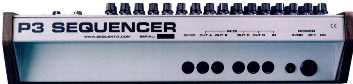
As befits a hardware sequencer, the P3 has four MIDI Out sockets to its one MIDI In. There's also a DIN Sync socket (the leftmost DIN socket) for connection to old Roland gear that uses this pre-MIDI sync protocol.
