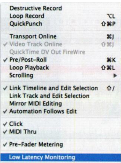
With the 002 and 002R, Pro Tools LE offers a special Low Latency Monitoring mode.
