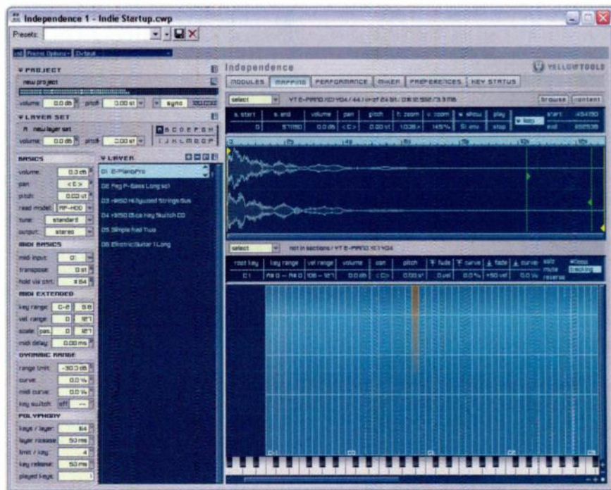
Mapping View, including the waveform of the currently selected Zone, with its start, end and loop points. The Zone's velocity crossfade area can be clearly seen.
