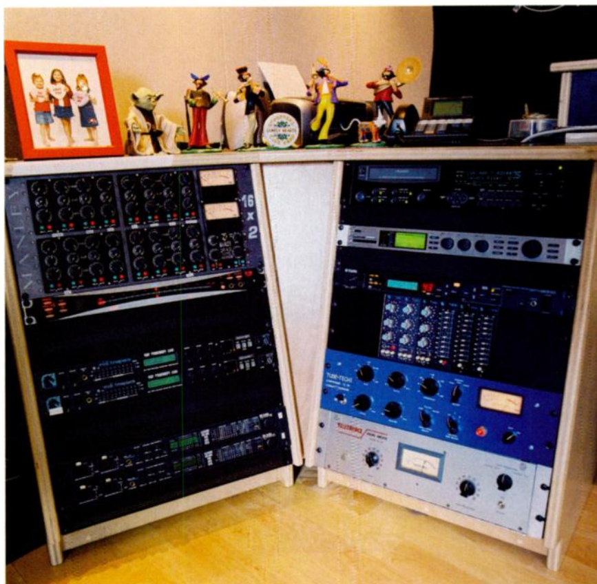
Some of the rackmount gear at Phantom Studios. Left, from top: Manley line mixer, MOTU MIDI Timepiece synchroniser (x2), MOTU 828 interface (x2). Right, from top: Alesis Masterlink CD master recorder, TC Electronic Fireworx effects, Yamaha SPX200 effects, API parametric and graphic EQs, Tube-Tech CL1B compressor and Teletronix LA2A compressor.
