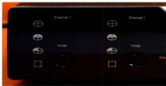
Four status indicators on the front of the amplifier show the settings of the internal DSP filter bank.
