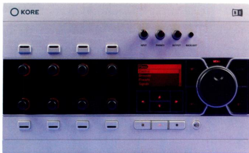
The Kore controller's rotary knobs are infinite encoders, which always reflect the position of the assigned parameter.
