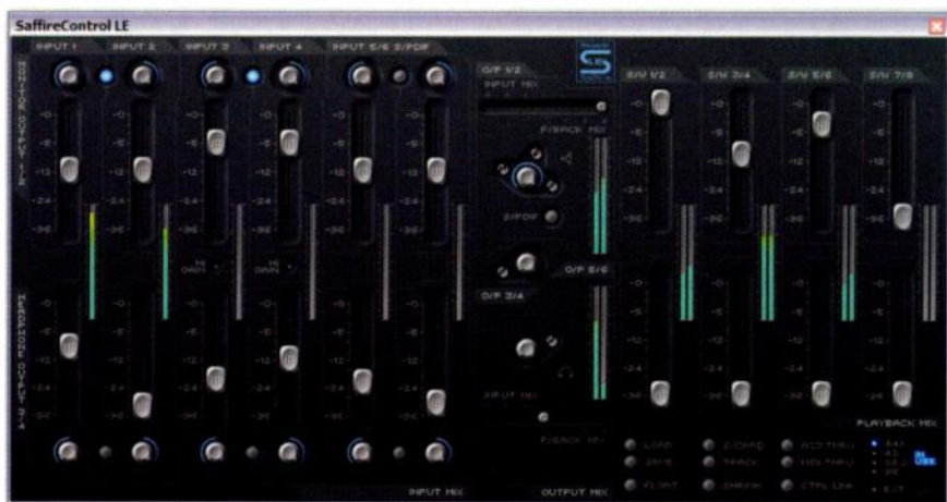
With comprehensive monitor mixing and metering of input and output levels, the Saffire LE's new Control utility is effective across a variety of recording and playback scenarios.
