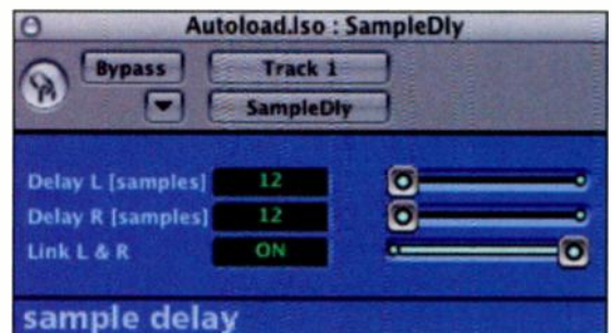
The Sample Delay plug-in in Logic does what it says on the tin, delaying the track down to sample level.
