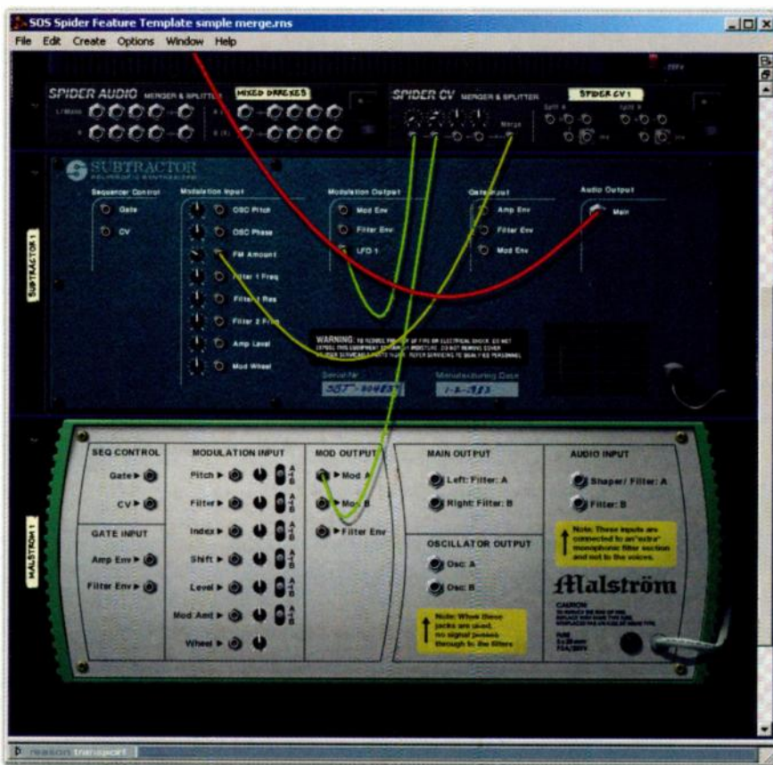
Here, the Malstrom is providing an extra modulator for Subtractor , but it's being mixed with the Sub 's own LFO1 output, creating something more complex with a simple cabling setup.
