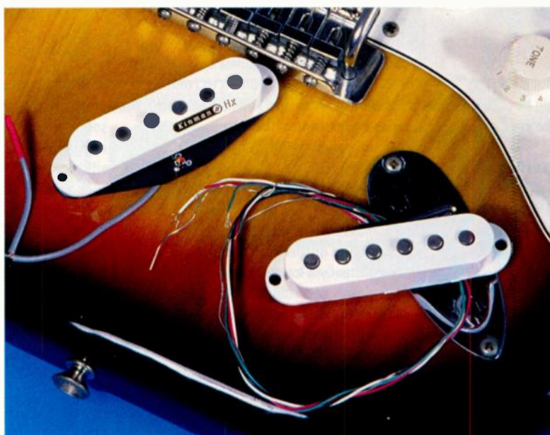
'Noiseless' single-coil pickups, such as these models from Kinman and Dimarzio, will cancel hum effectively, but noise can still get into the system via the wiring and controls.
