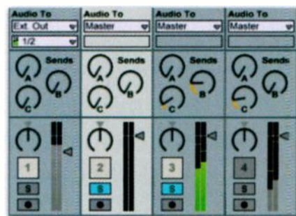
Tracks one, two, and three are activated, four is not. Tracks two and three are soloed, so track one's activate button is greyed out. Note that its meter is also grey.
