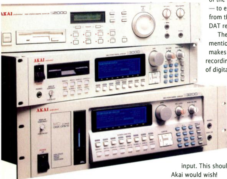
Akai's digital output-equipped sampler range featured a DAT backup and restore function.
