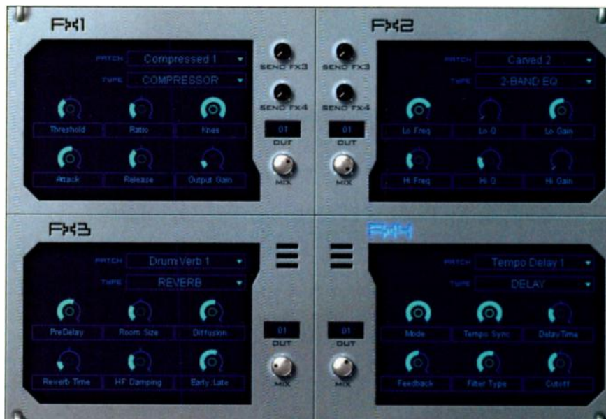
One's four internal effects units. The top two provide insert effects, while the bottom two offer send-return treatments.
