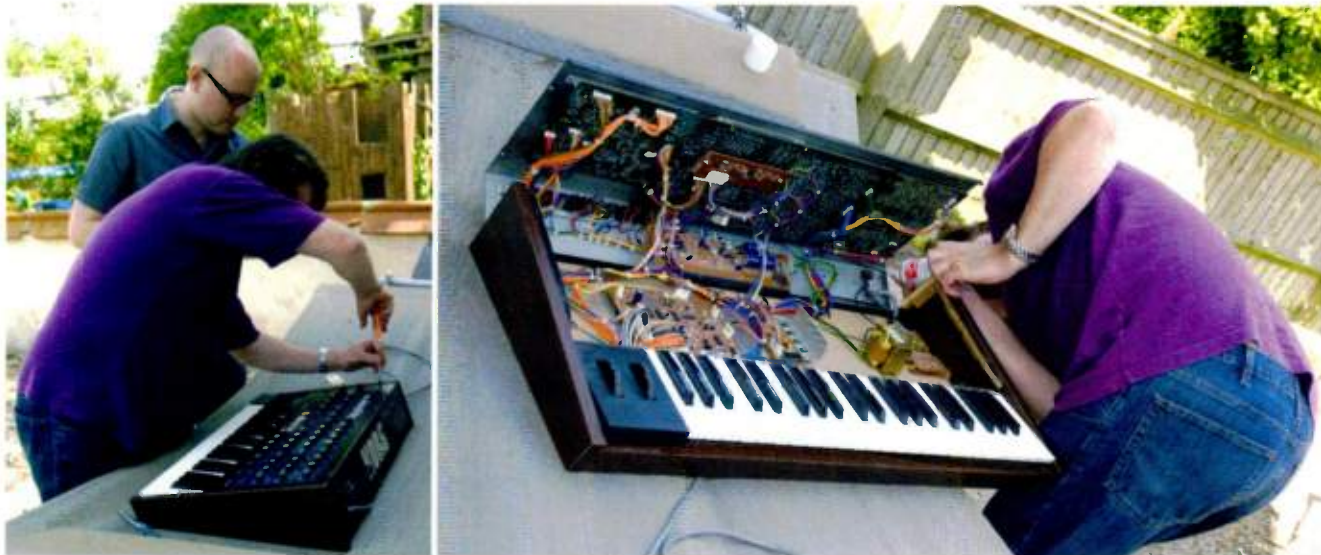
Banishing the crackles from a couple of pots on an old Korg Mono Poly involved just removing a couple of screws to whip the top open and then squirting a little contact cleaner into the underside of the offending controls.
