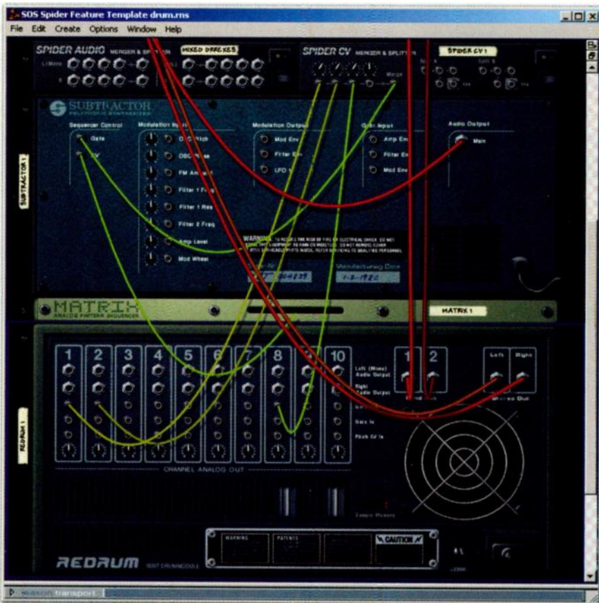
The gate outs of three Redrum voices, which are happily playing their own parts, are merged to provide the triggers for a Subtractor , which is deriving pitch information from a Matrix . The Matrix is folded because my screen wasn't big enough to show the whole example!
