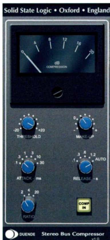
Dynamics processing used on the main mix buss comprised SSL Duende's Stereo Bus Compressor and Waves L1 Ultramaximizer .
