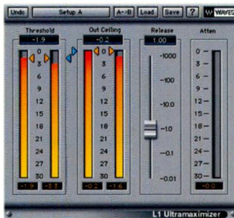
Dynamics processing used on the main mix buss comprised SSL Duende's Stereo Bus Compressor and Waves L1 Ultramaximizer .
