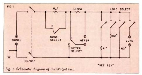
resistor, which can be switched into the signal path for current mode, or switched out for voltage mode; a multiposition switch to select one of several calibration resistors, or the test load; the calibration resistors; a precision current shunt; a switch for the meter to read either voltage or current. In addition there should be a switch to disconnect the signal source, and of course connectors for signal, meter, and load.
