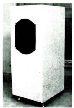
satisfactory for me. I opted to increase the internal volume so that the -3dB point be lowered to 38-39Hz in order to obtain a flat response of 41-42Hz, and still have Q around .7. The internal volume was increased from 3800 cubic inches (2.19 cu. ft.) to 5170 cubic inches (2.99 cu. ft.) in each box. The final total figure takes into account the displacement of volume by the driver, bracing, and damping material used for each panel wall. The effective internal
