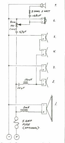
Fig. 2b. Crossover network schematic. See text.
