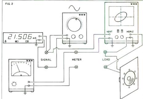
Fig. 2. Test setup using the Widget. The six crossed terminals in Fig. 1 are represented by the six crossed terminals above. The box interconnects meter, frequency counter, audio generator, oscilloscope and driver.
