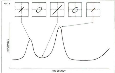
Fig. 3. A typical resonant peak pattern of a driver and the oscilloscope patterns indicating various nodes.
