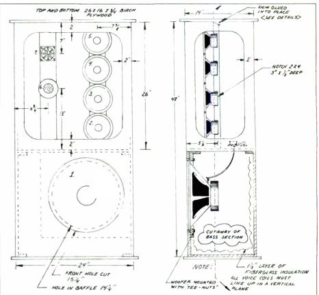
Fig. 1. Front and side views of the Model VII. Drawings by the author. Note the alignment of the voice coils of all drivers. Speaker units should be mounted in mirror image fashion for left and right versions. Woofer is off center to avoid diffraction.
