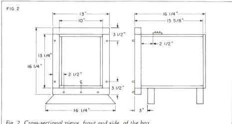
Fig. 2. Cross-sectional views, front and side, of the box.
