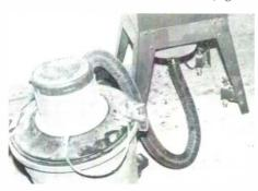
Fig. 8. Vacuum attachment for the table saw.
