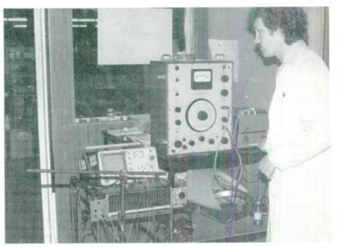
Fig. 17. Richard Ramsey does the "cloning" test where the production line model is tested against a measured standard speaker using a square wave, inverted in one and both equidistant from a probe mike. A good speaker "cancels" the standard one.
