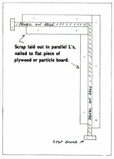
FIGURE 3: You can make a quick-and-easy jig out of scrap for assembling speaker cabinets.
