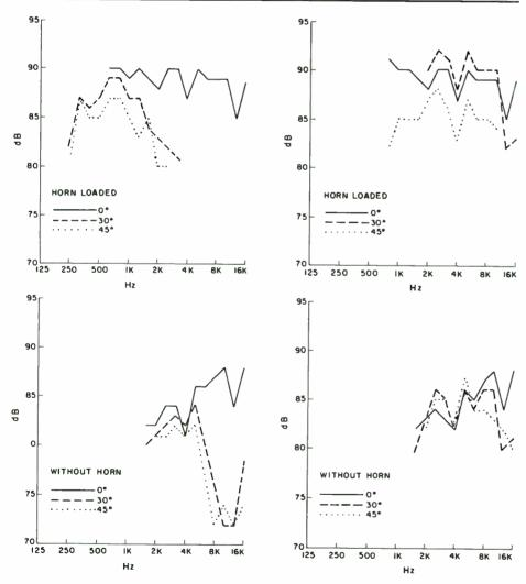
FIGURE 5: Vertical dispersion frequency response curves for the 3.7:1 diaphragm (with the first enclosure enlargement) shows the effect of horn loading is to transpose the curves downward. Very little coloration is added by the horn.
