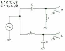
FIGURE 4. A second order parallel filter requires two coils.
