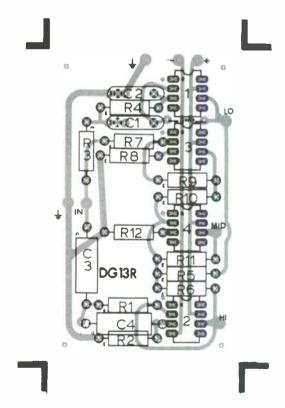
FIGURE 2b: Layout guide for DG-13R board.
