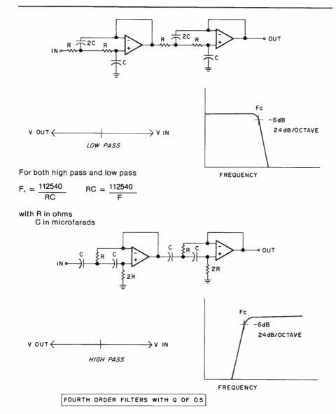
FIGURE 2. In fourth order filters, a very sharp rollover slope occurs, and the high and low pass outputs are in phase with each other.
