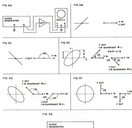
FIGURE 6. Testing phase angle requires only an oscillator and an oscilloscope. When the scope shows the patterns in B and C, phase shift is 0 and 180 degrees respectively. In D and E, the ellipse has poles in two quadrants, so to determine whether phase shift leads or lags, use a "phase reference circuit" with known shift, as shown in G. Leading phase will show a circle as in F, lagging phase, a straight line.
