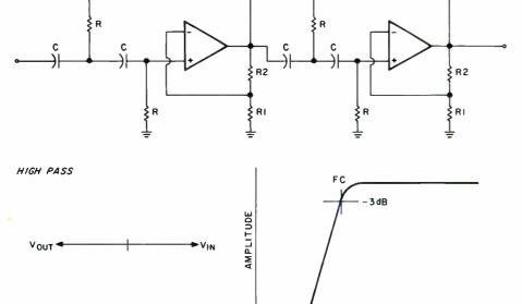
FIGURE 3. By changing the values of resistors (R, and R,) the Q (resonance) of the filter can be altered.
