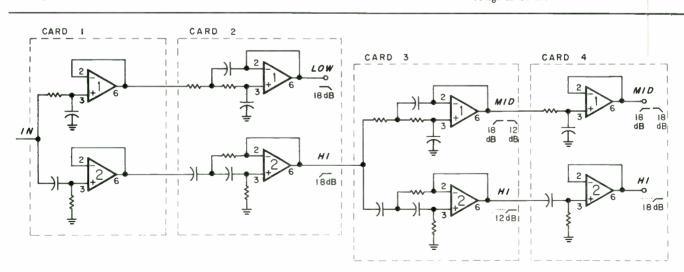
FIGURE 5: Three-way, 18dB per octave utilizes four single channel boards for one audio channel. Boards I and 4 omit R<sub>2</sub>, C<sub>1</sub>, R<sub>4</sub> and C<sub>4</sub>. Install jumpers in place of R<sub>4</sub> and C<sub>5</sub>. Choose one frequency for cards I and 2, the second frequency for cards 3 and 4.
