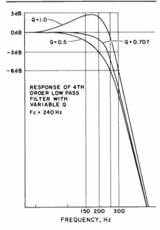
FIGURE 4. Changing the Q alters the response curve. When Q = .707, the curve extends further along the OdB line than for any other value, or is "maximally flat."
