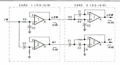
FIGURE 4: 18dB/octave, cascaded, two-way crossover, one channel use jumpers in place of  $R_4$  and  $C_4$ . Omit  $R_7$ ,  $C_1$ ,  $R_4$ ,  $C_4$ . Frequency determining elements are the same for both cards.
