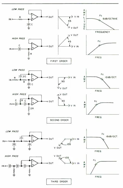
FIGURE 1. The phase and frequency response of first, second, and third order filters all have undesirable characteristics. Phase delay occurs when the phase vector rotates clockwise from  $\mathbf{V}_{IN}$  to  $\mathbf{V}_{OUT}$ . None of the three has an output with the high and low pass in phase with each other.
