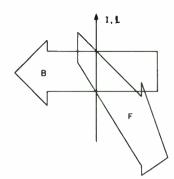
FIGURE 1: When current flows in a conductor it creates a magnetic force 90° from the direction of current flow, which is the operating principle behind all electromagnetic devices.
