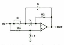
FIGURE 5. An all pass filter makes a good phase shifter. By using a variable resistor for R, the phase shift can be adjusted as desired.
