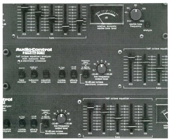
The Richter Scale ™ is the world's first half-octave bass equalizer with built-in electronic crossover, Rumble Reduction ±1dB 20Hz-20,000Hz. Circuit, 18dB/octave Subsonic Filter,
