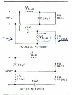
General use of "constant impedance" networks is not good because of the impedance variations in individual speakers. They can be used over a frequency range where the driver behaves (or is made to behave) as a resistor. For an example of how this works, look at the two networks in Fig.1, which are se-
