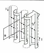
FIGURE 2: In the Heil driver, the magnetic field is oriented from front to back. As current flows through the conductor, the pleats are squeezed together on one side, and spread apart on the other.
