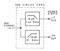
FIGURE 7a (above): Two-way, single channel crossover using one WJ-3 (F-6) board.
