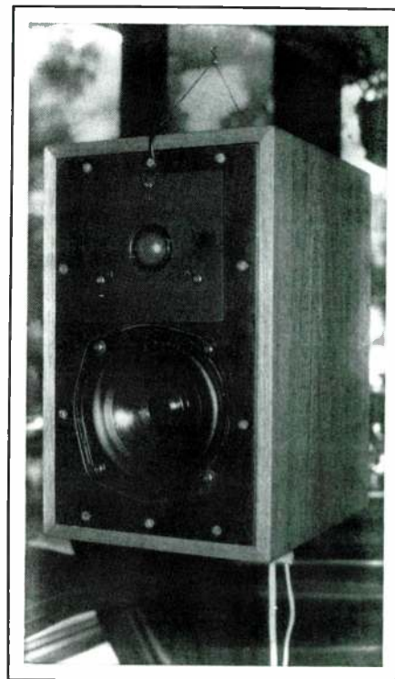
PHOTO 2. The satellite speakers are small enough to be suspended from the ceiling. Damped with long hair wool and coated internally with bitumen, they use Dynaudio dome tweeters, and KEF midranges.
