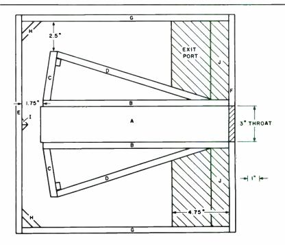
FIGURE 12: This side view shows the placement of parts and the critical dimensions.
