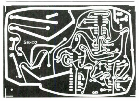
FIGURE 12: Circuit board pattern for the pulse generator.
