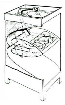
FIGURE 3: RCA's Orthophonic phonograph of 1926 used a folded horn and inspired Edgar's design.
