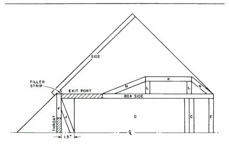
FIGURE 14: This top view of one half of the box module shows the location of the outer flare pieces.
