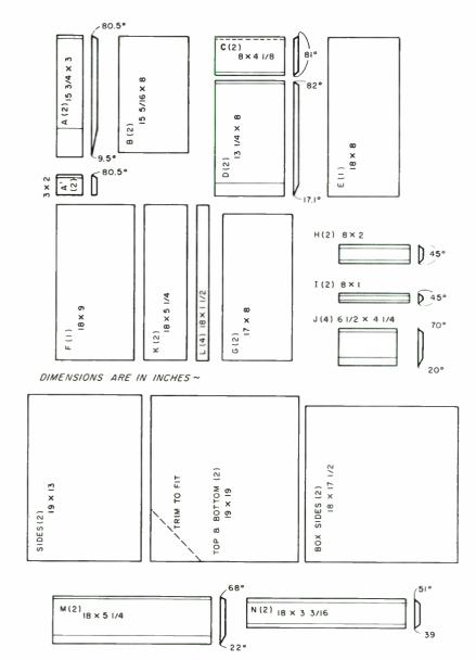
FIGURE 5: The dimensions for all of the particle board parts are as shown. The number needed for one complete horn is circled inside each part.
