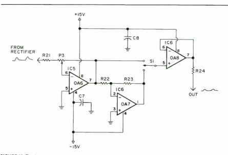
FIGURE 10: The level amplifier uses an inverting op amp (OA6) with variable gain. OA7 is another inverter, and the switch selects positive or negative pulses.
