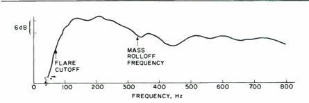
FIGURE 19: System response with the mid-size box extends down to 70Hz.
