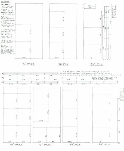
Figure I: Cutting guide for bass enclosure.
