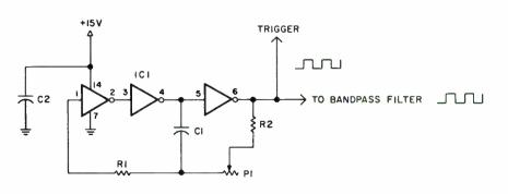
FIGURE 7: The schematic for the clock is a square-wave oscillator built from three inverting buffers.
