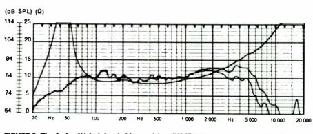
FIGURE 2: The Audax 6½-inch bass/midrange driver (HD17B25H) curves on axis and 30° off axis, plus its impedance curve.
