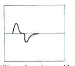
FIGURE 4: If the manufacturer has reversed the polarity between the two drivers, the pattern on the scope looks like this.
