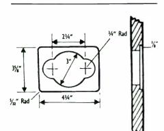
FIGURE 4: Cutout details for the tweeter mounting. Note the ¼-inch recess, which allows you to flush mount the unit's steel plate.
