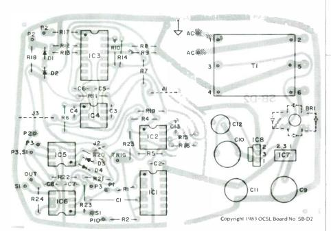
FIGURE 13: This is the stuffing guide for the SB-D2 circuit board. Note that the transformer T1 has a spare set of holes near the board's edge for a slightly larger board mounted transformer. The author's Signal PC 34-125 fits the closer holes. Signal's PC 34-300 fits the wider ones. BR-1 is a standard full wave bridge, which fits the inner four holes. Extra holes are provided if you prefer to use less expensive IN4001 diodes.
