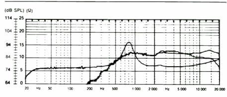
FIGURE 1: The Audax 1-inch tweeter response curves on axis and 30° off axis, as well as its impedance curve.
