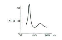
FIGURE 18: With the mid-size box, the resonance is at the right place for smoothest overall response.
