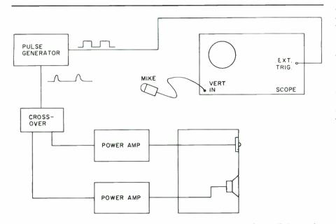
FIGURE 3: After passing through the crossover and the drivers, the pulse as picked up by the mike has two time components. The pulse from the woofer is behind the one from the tweeter.
