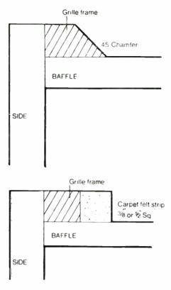
FIGURE 6: Grille frame construction details show methods of either beveling the inner edge or adding jute rug pad material to diminish diffraction problems.
