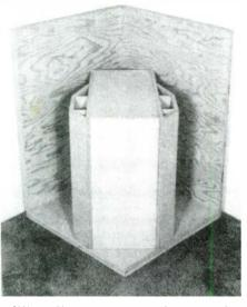
FIGURE 16: Use a temporary corner jig of plywood to align the top and bottom pieces.
