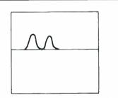
FIGURE 5: After rewiring the drivers for the same polarity, adjust the pulse frequency so the amplitudes are equal.
