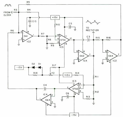
FIGURE 8: The schematic for the bandpass filter shows how OTA's instead of resistors provide variable center frequency.
