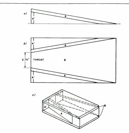
FIGURE 8: Begin construction with the throat manifold. The three steps in its assembly are illustrated above.
