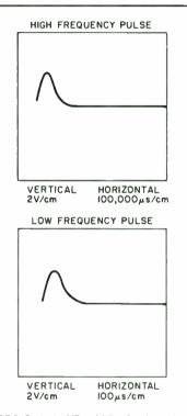
FIGURE 2: Both the HF and LF pulses have the same shape and polarity (positive shown above).
