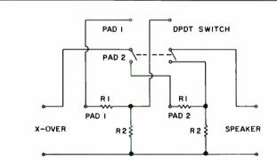
FIGURE 3: Simple switchable L-pad.
