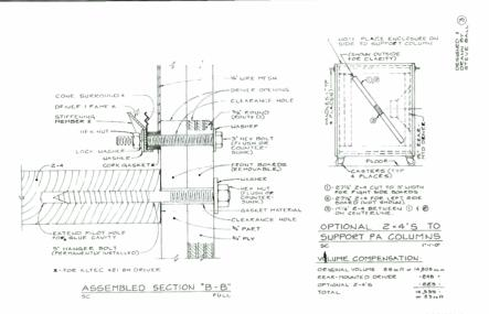
Figure 2: The author designed this enclosure for a 15-inch Altec driver to be driven by a 300W/channel McIntosh. This accounts for the extra-thick wood and additional bracing.
