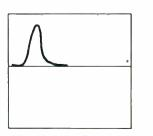
FIGURE 6: When the drivers' outputs are in phase acoustically, the pulses in the scope overlap and have maximum amplitude.
