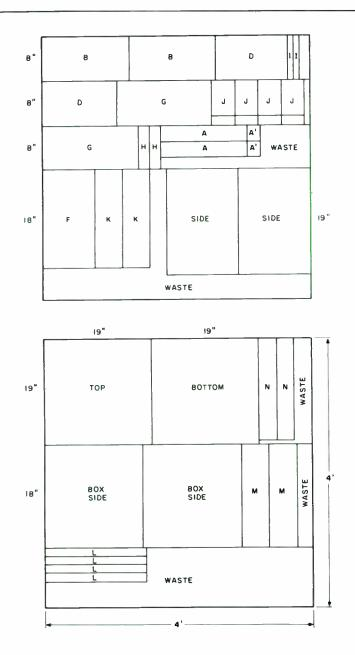
FIGURE 6: For efficient use of the %'' plywood or particle board, cut the parts with this pattern.
