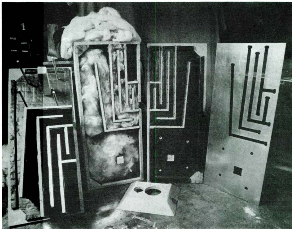
This photo, taken by Harold Holden, shows the transmission line in the making. The shiny lead sheet at the right functions as a template as well as effective resonance damping.
