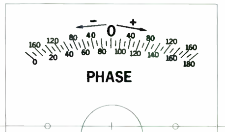
FIGURE III-13: Phase meter scale for the meters discussed in this article. Do not scale for use on other meters.
