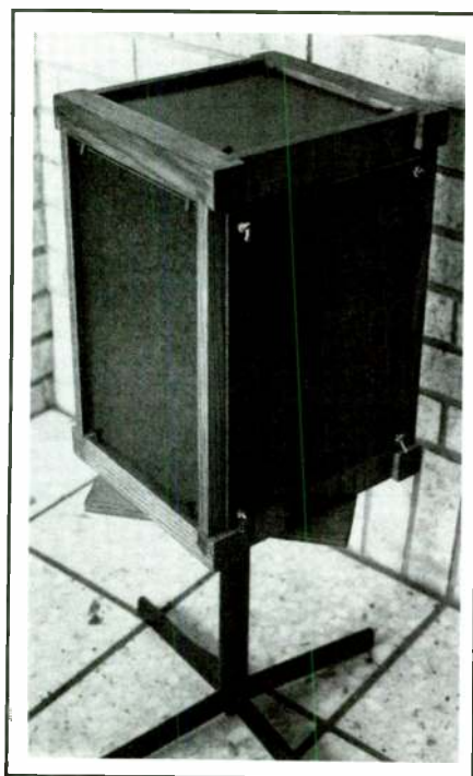
FIGURE 3: This speaker has hardboard instead of plastic sides. The sides must not touch the frame or they will rattle.
