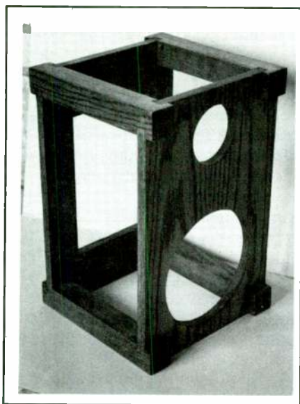
FIGURE 2: The front and back of the speaker frame are made of \frac{3}{8} -inch solid oak, but plywood will work as well. The four struts connecting the back and front are made of 1\frac{1}{4} -inch oak.
