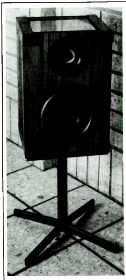
FIGURE 1: A front view of the author's speaker design with clear plastic sides attached.
