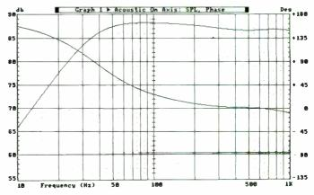
FIGURE 1: AC-10, 1W/88, dB/25, C - 3dB phase angle 92.8.
