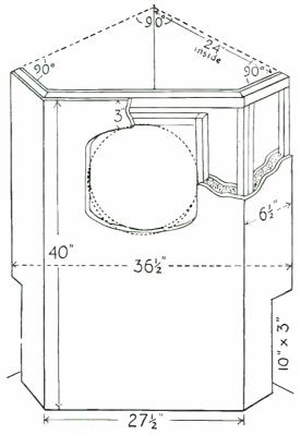
Distance along wall from corner to front of lid is  $26\frac{1}{4}$ " Weight of front panel 124 lb.
