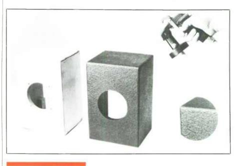
Texturelac, new from ARD, is a paint product designed for speaker cabinets that gives a spray finish that looks like pebbles, stucco or leather. The different patterns are created by adjusting air and fluid pressures using standard Binks and DeVilbiss guns.
