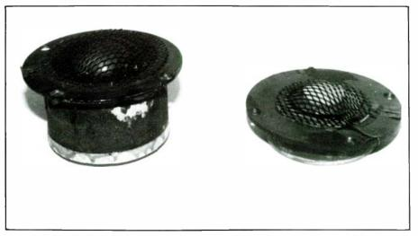
PHOTO 3: The AR-3 midrange (L) as compared to the AR-3a midrange (R).
