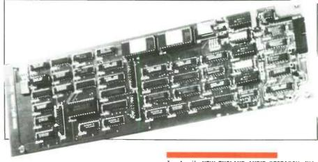
The R712, from **RAPID SYSTEMS**, is a multifunction analog/digital I/O card for the PC, XT, AT, or compatible computer. This card offers 12-bit resolution in both A/D and D/A conversion. Also on the card are a three-channel programmable interval timer/counter, and 16 digital inputs and outputs. Sample programs are included with the user manual and controlling software is available.
