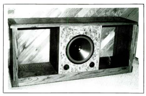
PHOTO: Back of the credenza and rear-firing subwoofer.
