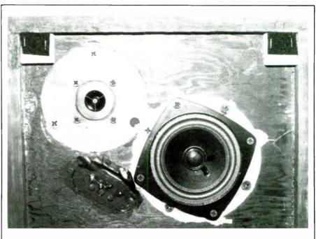
PHOTO 10: The Peerless KO40MRF and Audax TW51A units installed in the AR-3 box.
