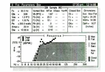
Introducing BassBox", the bass loudspeaker enclosure design program for IBM PCs. With it you can quickly determine the optimum enclosure size and tuning for a given loudspeaker or examine the response of various loudspeakers in an existing enclosure. Both vented and sealed enclosures can be modelled and their dimensions found.
