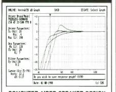
**COMPUTER-AIDED SPEAKER DESIGN** CASD allows the design and modeling of vented, closed and passive radiator systems based upon the Thiele/Small model. The program also allows the use of equalization filters for B6 alignments. CASD includes a user modifiable driver database of over 750 drivers for powerful searches and sorts. Other features include nine utilities and Butterworth crossover designs.
