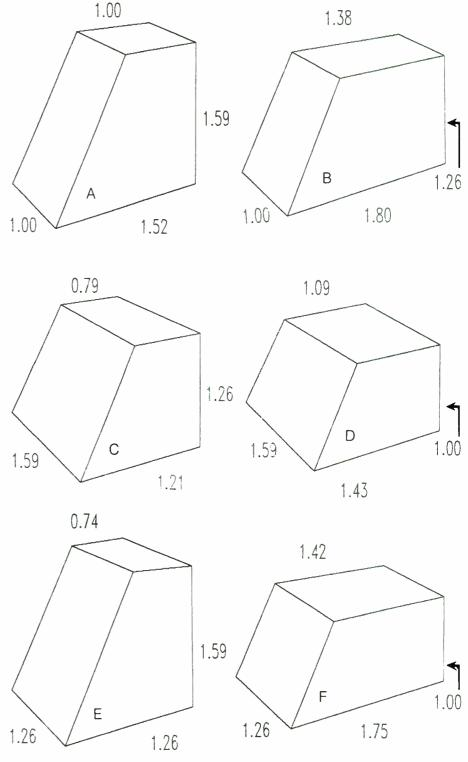
FIGURE 2: Slanted-front enclosures. The drivers are mounted on the panel shown on the left side of the drawing.
