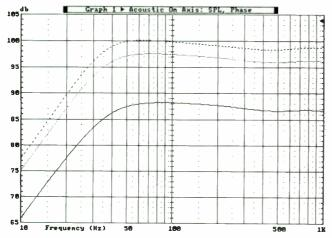
FIGURE 5: AC-10, 1W/88, dB/25, C - 3dB at phase angle of 92.8.; 10W/98, dB/50, C - 3dB phase angle 97.4; and 20W/100, dB/75, C - 3dB, phase angle 101.1.
