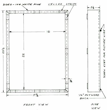
FIGURE 1: Absorber frame construction.
