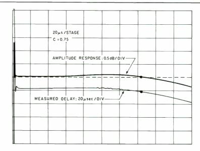
FIGURE 5: Measured response of four cascaded  $20\mu$ sec-delay sections (C = 0.75).
