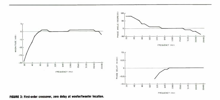
whose phase angle approximates that of an ordinary time delay. By physically displacing the tweeter (via the unusual slanted front baffle), its own time delay relative to the woofer matches that approximated by the Bessel filter. Thus, both drivers are approximately equivalent to a single driver with a time delay.
