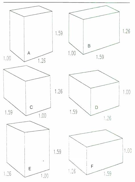
FIGURE 1: Simple rectangular enclosures. The drivers are mounted on the panel shown on the left side of the drawing.
