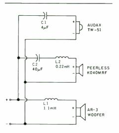
FIGURE 2: The new 6dB crossover for the modified AR-3.
