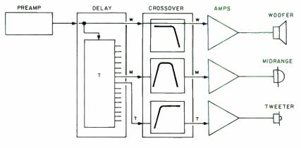
FIGURE 8: Preferred installation location of delay line.
