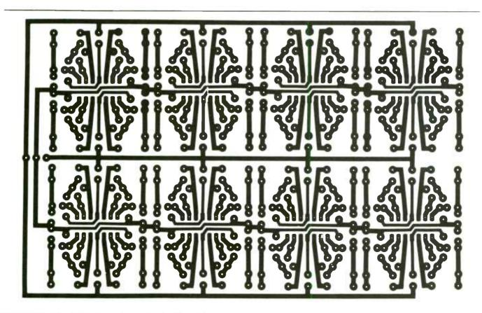
FIGURE 6: Circuit board for two channels of 320µsec maximum delay.
