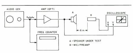
FIGURE 10: Setup for measuring relative acoustic centers of drivers.
