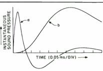
FIGURE 1: Step response of tweeter (a) and midrange (b) models with ideal third-order crossover.
