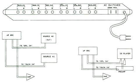
FIGURE 1: The back of the AR-SRC and typical SUT/reference comparison connections.
