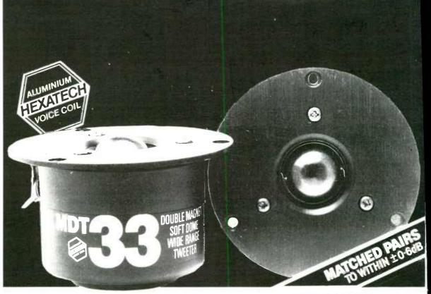
The MDT 33 is an extremely fast Tweeter, using a 28mm (1 1/8 ") diameter voice coil and a chemically treated soft dome, and is ideally suited for two way systems with the possibility of a lower than normal crossover frequency, as well as for three and multiple way systems.
