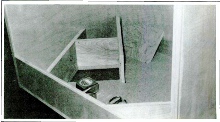
PHOTO 7: Trying a trial compound angle for the corner reflector J. Note: The throat opening, shown cut on a temporary top piece, is for experimentation purposes.
