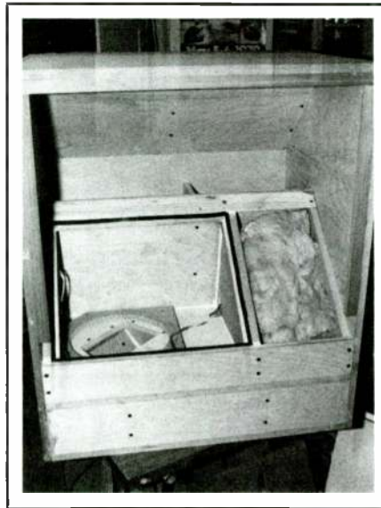
PHOTO 10: Finished back chamber with speaker mounting board.
